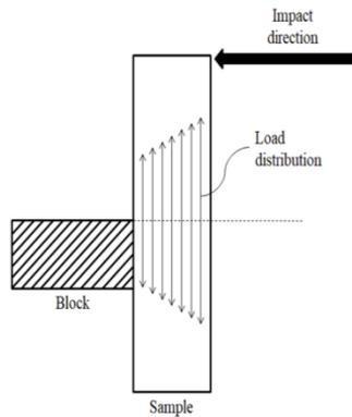
**Figure 6.** Schematic diagram of load distribution during impact test.
