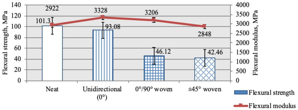
Figure 3. Average values of flexural strengths and flexural moduli of sugar palm fibre reinforced VE composite
