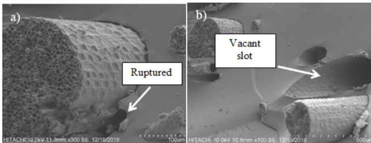
**Figure 9.** SEM of  $\pm 45^\circ$  woven fibre VE composites showing some flaws i.e. a) ruptured matrix and b) vacant slots
