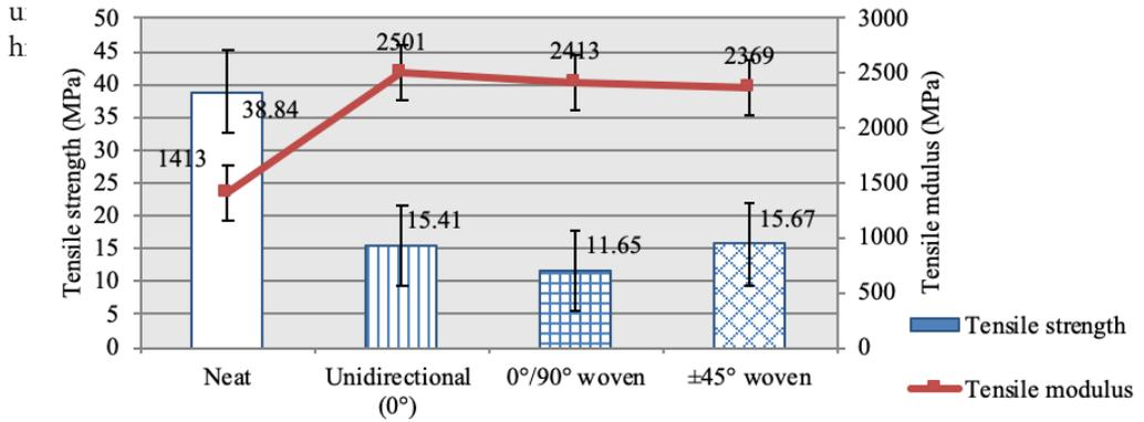
Figure 2. Average data of tensile strength and tensile modulus
