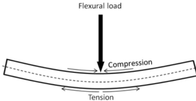
Figure 4. Schematic diagram of flexural stress distribution
