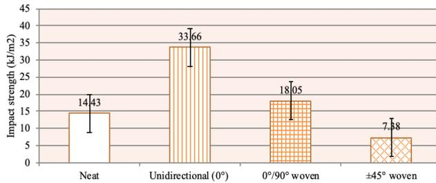
**Figure 5.** Average results of impact strength of sugar palm fibre reinforced VE composites at different fibre arrangements
