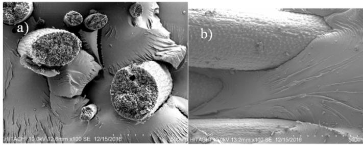
**Figure 8.** SEM image of 0°/90° woven VE composites with a) fibres in vertical direction and b) fibres in horizontal direction
