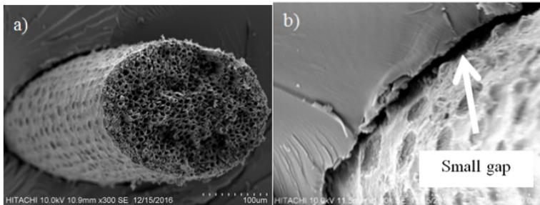
**Figure 7.** Occurrence of a) broken fibre, and b) small gap; of fractured surfaces of samples in impact test (SEM image)
