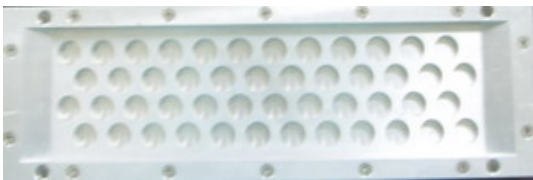
Stainless steel mold with diameter of 16 mm.
