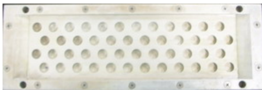
Stainless steel mold with diameter of 12 mm.
