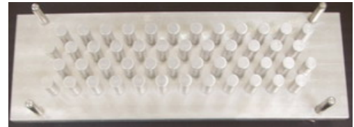
Stainless steel mold with diameter of 12 mm.
