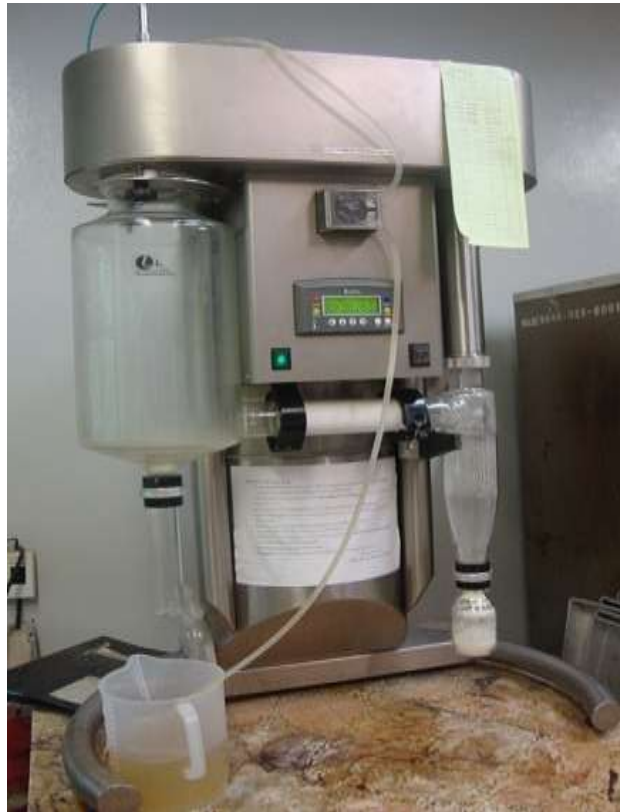
Figure 8 Spray dryer (Model: SD-06 Brand, Lab Plant Ltd, England)
