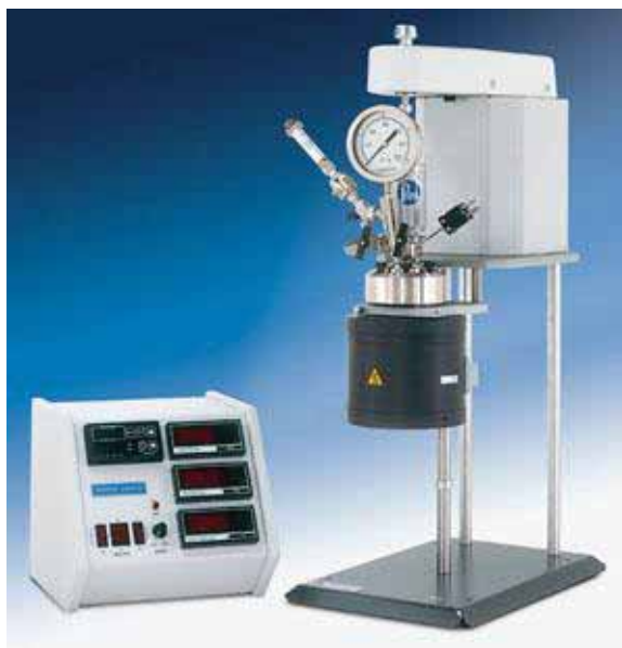
Figure 4 Autoclave for support preparation (Parr Instrument 2009)
