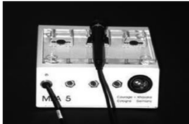
Figure 2.7 The MPA5 the main unit of Corneometer 825
