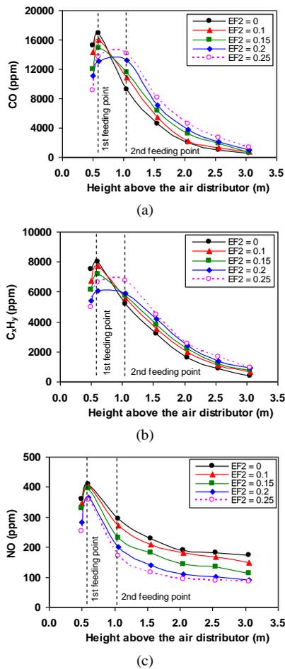
Figure 3. Effects of the energy fraction of secondary fuel ( $EF_2$ ) on the axial profiles of (a) CO, (b)  $C_xH_y$  (as  $CH_4$ ), and (c) NO in the conical FBC (co-) fired with PRH and MRH in different proportions at constant excess air ( $\sim 40\%$ ).
