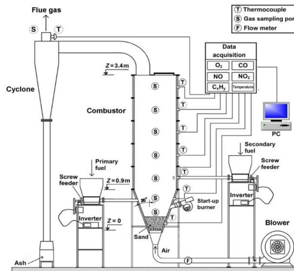
Figure 1. Schematic diagram of the experimental setup for fuel-staged co-firing of two biomass fuels.
