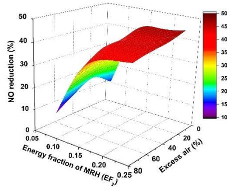
Figure 5. Effects of the energy fraction of secondary fuel ( $EF_2$ ) and excess air on the NO emission reduction of the conical FBC when using fuel staging, relative to baseline use of only the primary fuel.
