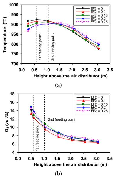
Figure 2. Effects of the energy fraction of secondary fuel (EF<sub>2</sub>) on the axial profiles of (a) temperature and (b) O<sub>2</sub> in the conical FBC (co-)fired with PRH and MRH in different proportions at constant excess air (~40%).
