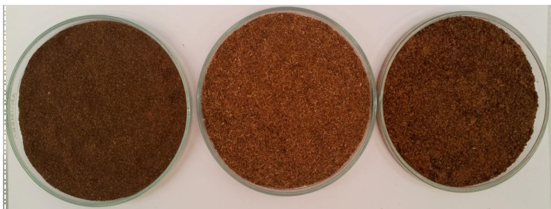
Figure 5.4 Comparing of DDF, FDF and Bleached DDF appearance after bleaching (from left to right)
