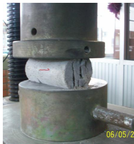
Figure 3.4 Test setup for splitting tensile test
