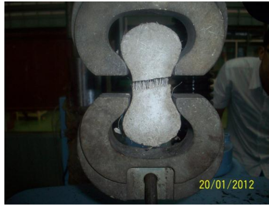
Figure 3.5 Test setup for direct tensile test
