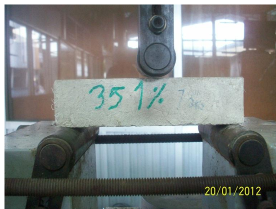
Figure 3.6 Test setup for measuring flexural strength of FRCC
