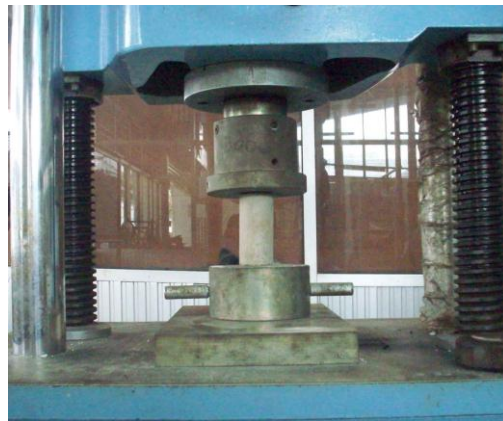
Figure 3.3 Test setup for compressive strength
