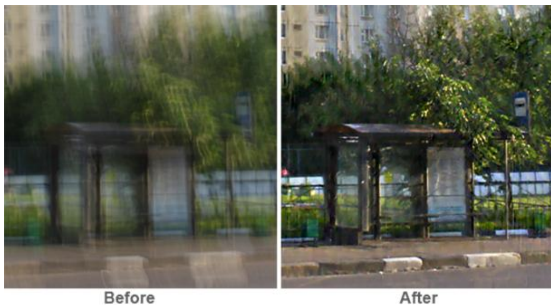
Figure 2.7 Corrupted image by motion blur is on the left and the restore image, on the right, is the result from motion deblur
