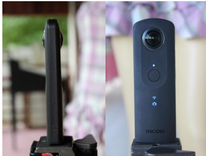
Figure 3.2 An example of a true 360-degree camera which uses 2 ultra-wide angle cameras to cover the entire 360-degree field of view
