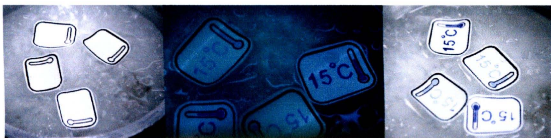
Figure 3.51 Polymerization of temperature indicating MPCDA screen ink in an ice bath.
