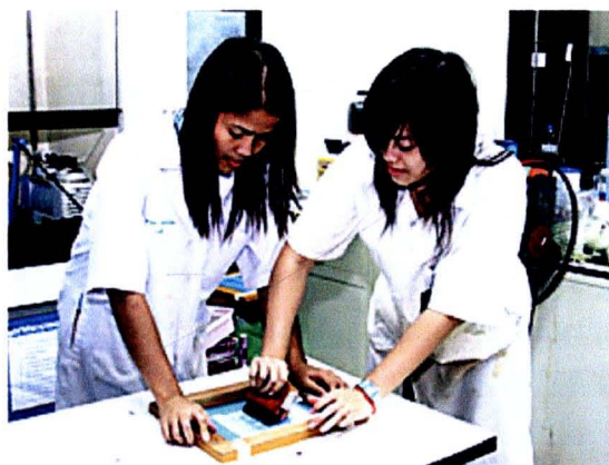
Figure 3.49 Screening of temperature indicating screen ink
