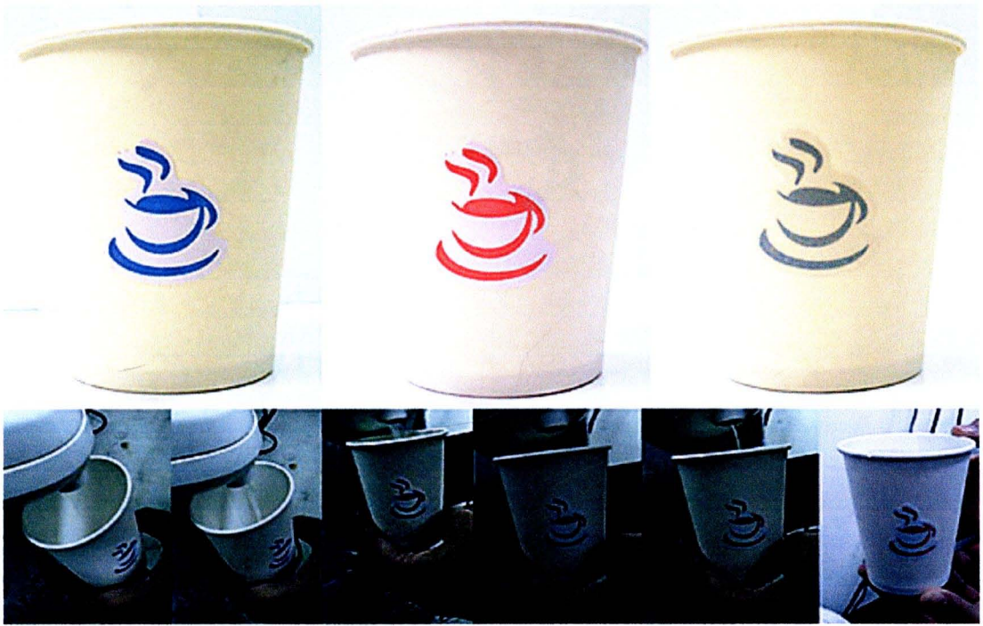
Figure 3.53 Using of temperature indicating label with hot cup. (left) PCDA label before given heat, (middle) PCDA label after given heat, (right) EBPCDA label, (below) Color changing of PCDA label during addition hot water.
