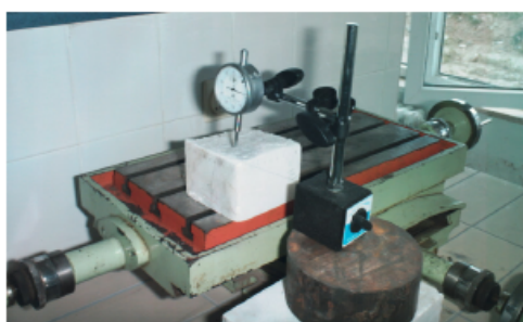
Measurement system by using dial gauge
