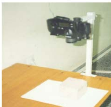
Taking stereo photo system for digital photogrammetry
