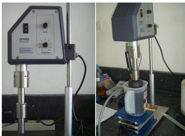
Figure 2.2 Equipment setup of the batch esterification
