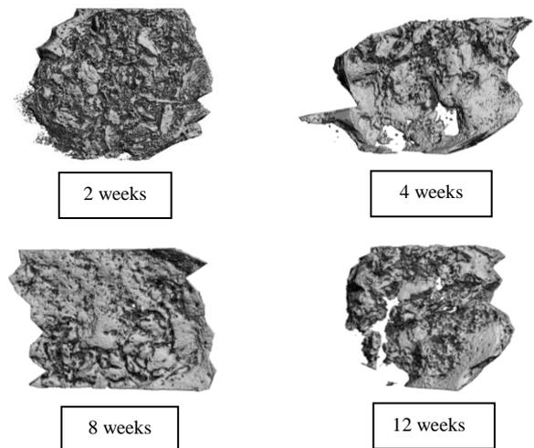
Figure 7. Micro-CT images of bone volume fraction of autogenous bone chip.
