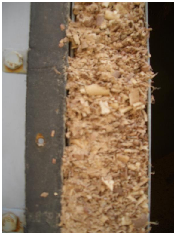
D7 Characteristic of wood dust inside panel filter
