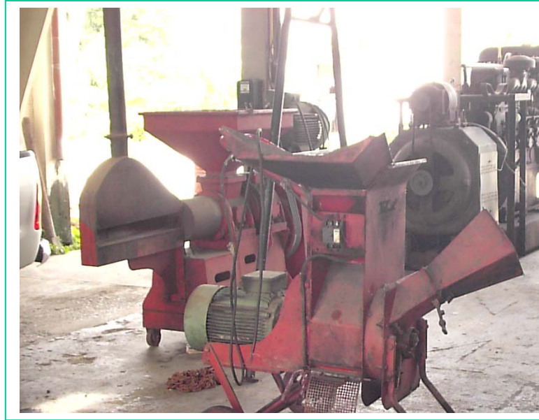
Figure B-1 Crusher machine
