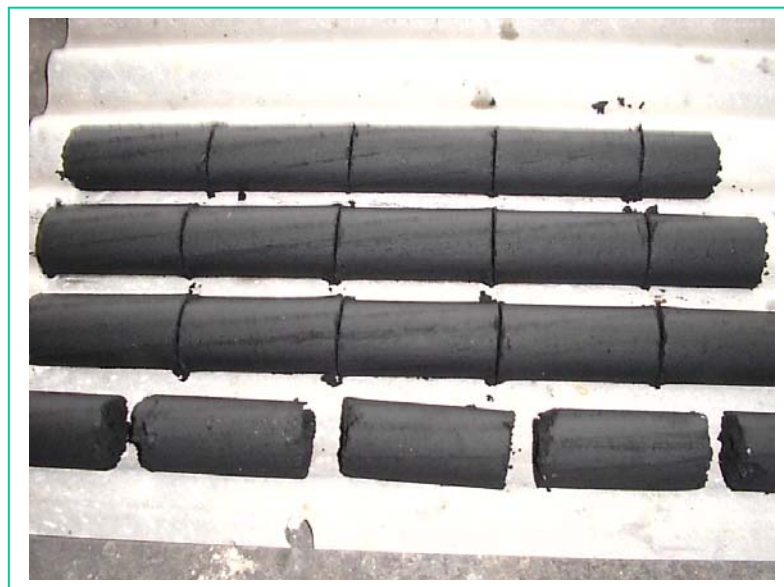
Figure B-9 Briquetted fuel product
