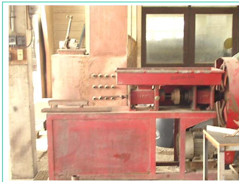
Figure B-2 The cold and low-pressure densification and the conical screw press
