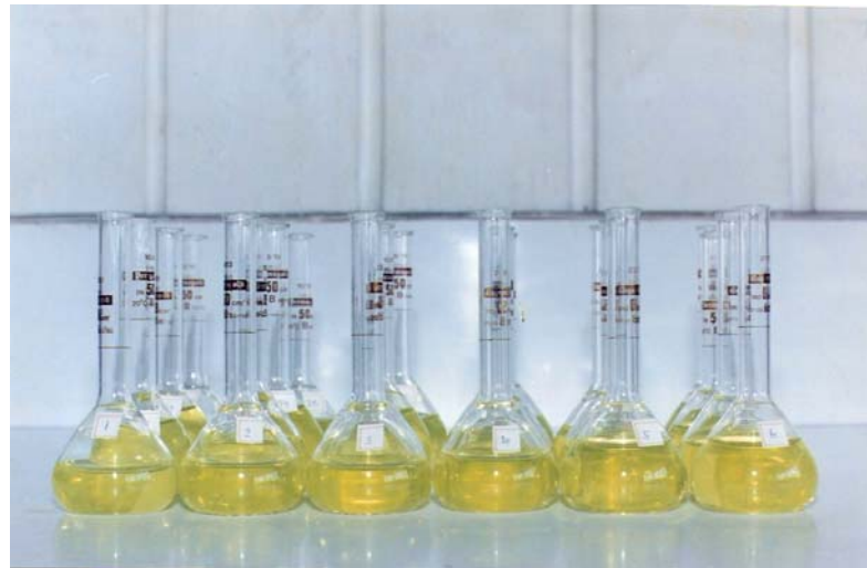
Figure 5B. After adding 1 drop of 1% paranitrophenol, slowly adding concentrated ammonium hydroxide until the sample turns yellow.
