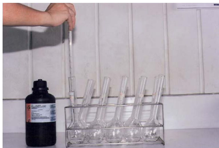
Figure 4B. Add 2 ml of 30 % hydrogen peroxide ( H_2O_2 ) into Kjeldahl flask .
