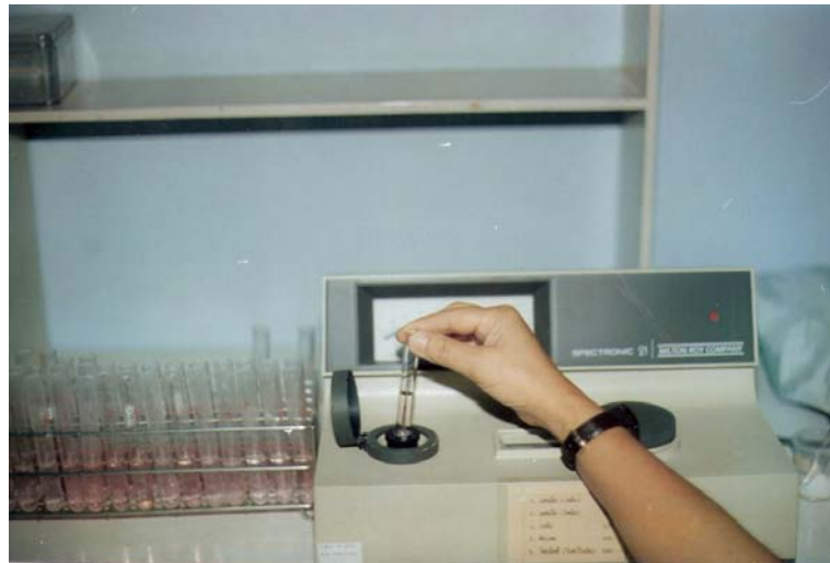
Figure 7B. The optical density was read in spectrophotometer at 535 nm.
