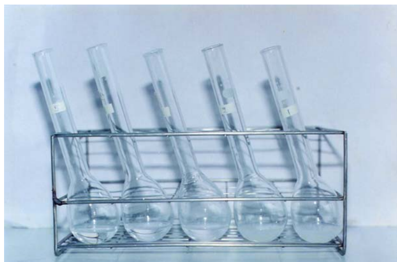
Figure 3C. Transfer the final eluted from column to Kjeldahl flask, added 0.5 ml concentrated sulfuric acid and 6.0 ml concentrated nitric acid to flask.
