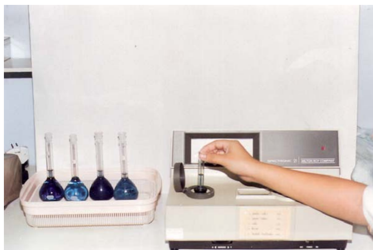
Figure 7C. The optical density was read in spectrophotometer at 640 nm after standing for 15 minutes at room temperature.
