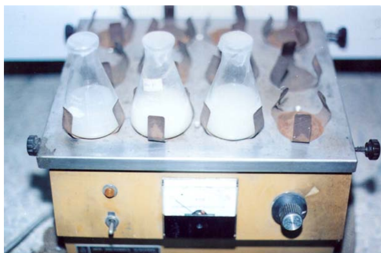
Figure 1C. Extract the food phytate with 2.4% HCl by shaking 3 hours at room temperature.
