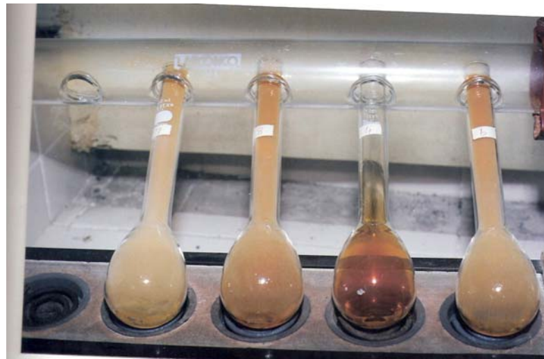
Figure 3B. Digest with low heat and gradually increase the heat until it becomes dark brown colour.
