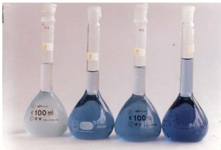
Figure 6C. The blue colour was developed according to the amount of phosphate after adding molybdate-sulfonic acid solution to the digested solution which transfers to 100 ml volumetric flask.
