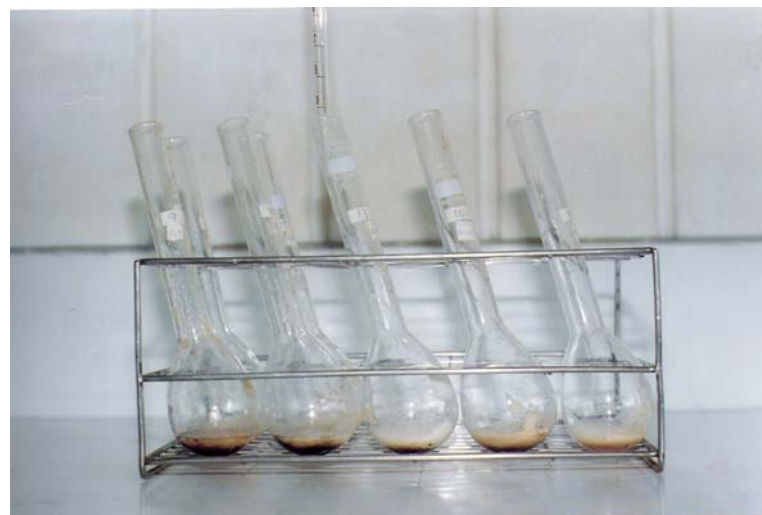
Figure 2B. Add 2.5 ml concentrated sulfuric acid and 2.5 ml concentrated nitric acid in to the Kjeldahl flask.
