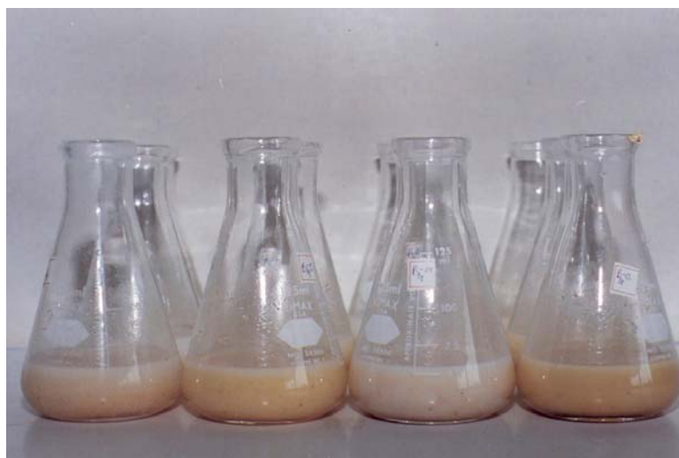
Figure 1A. Weaning food samples were incubated in water bath, 37 °C for 60 minutes after added 20 ml of 0.17 HCl, 5 ml of 1 % Pepsin and 500 \mu of Fe-59.
