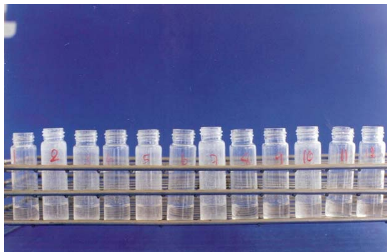
Figure 3A. Triplicate of 0.5 ml supernatant of digestion mixture was pipetted into 6 ml screw cap vials.
