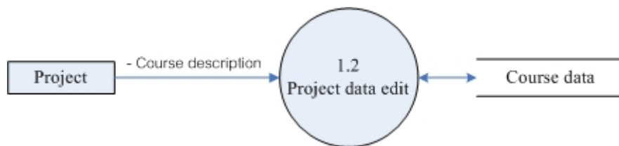
Fig. 4-4: DFD Level 2 Process II, Project and course data edited by searching and updating
