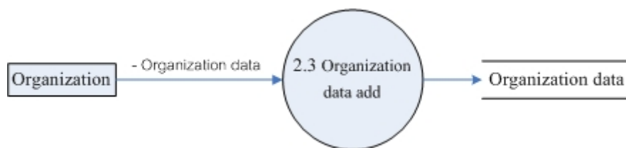
Fig. 4-11: DFD Level 3 Process III, Organization data adding into the database system.
