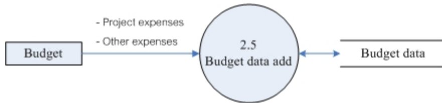
Fig. 4-13: DFD Level 3 Process V, Budget data adding into the database system.
