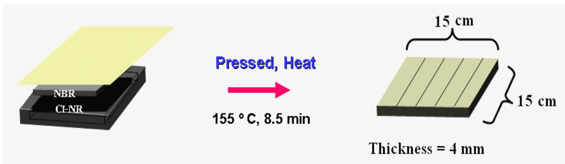
Figure 4.2 Preparation of NR//NBR sheet
