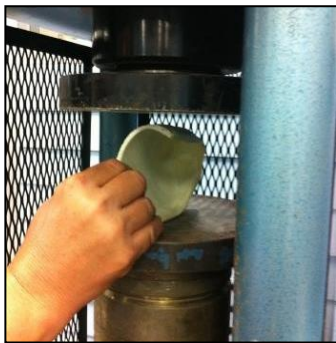
Fig. 3. Image depicting compression testing of the Scotchcast UCBL.
