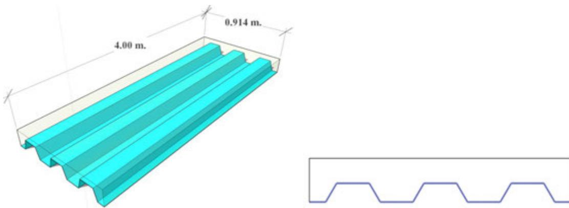
**Figure 5:** Details specimen SN of test performed by (Na-Lampoon, 2016)
