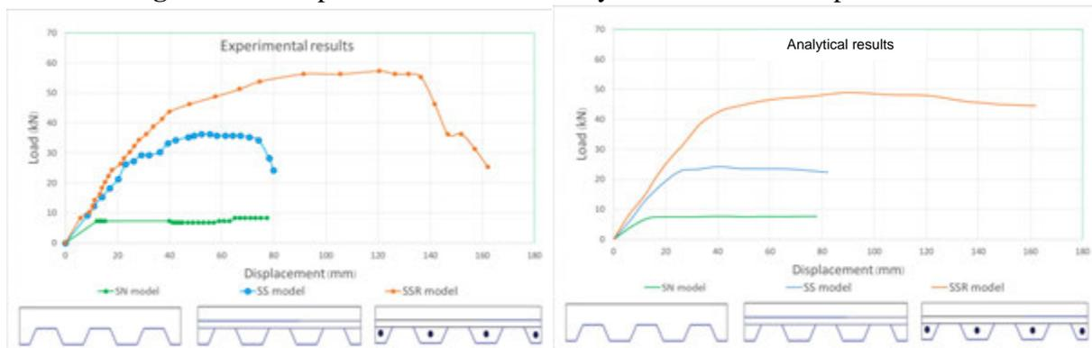
**Figure 12:** Test and analytical results of composite slabs.
