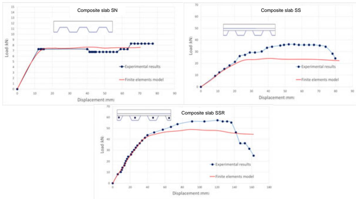
**Figure 11:** Comparisons of test and analytical results of composite slabs.
