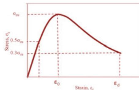
**Figure 2:** Compressive Stress-Strain Relationship for ABAQUS® by Hsu and Hsu (1994)
