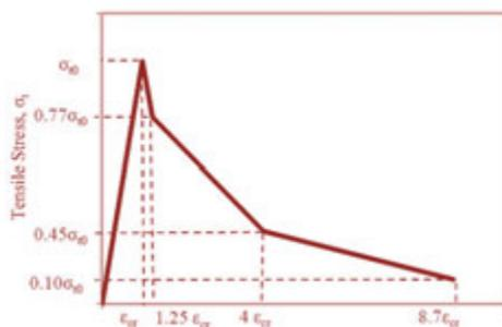
**Figure 1:** Tension Stiffening Model for Abaqus by Wahalathantri (2011).
