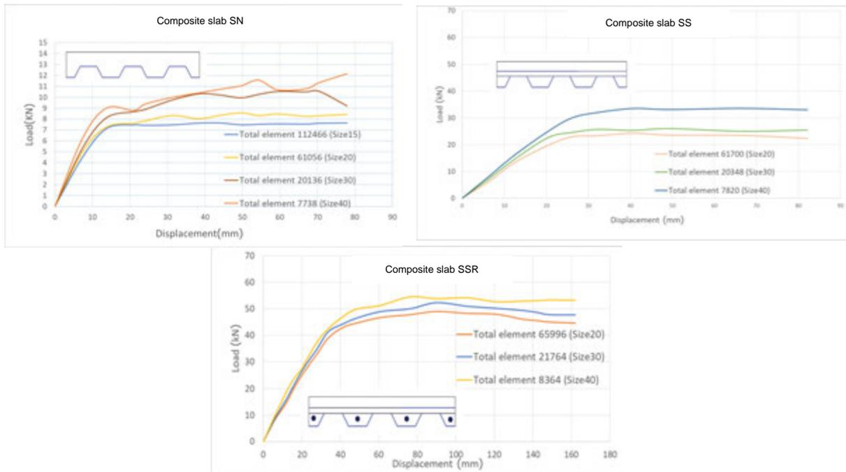
Figure 10: Mesh sensitivity on behavior under static loading of SN.
