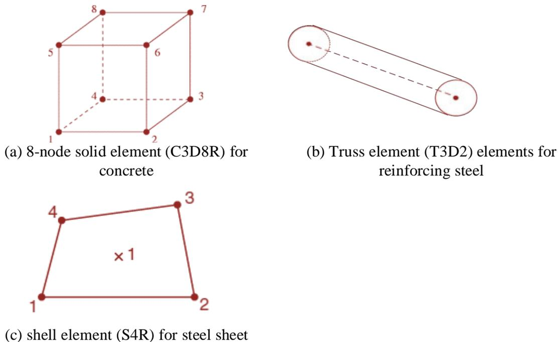
**Figure 4:** Element used in the finite element model
