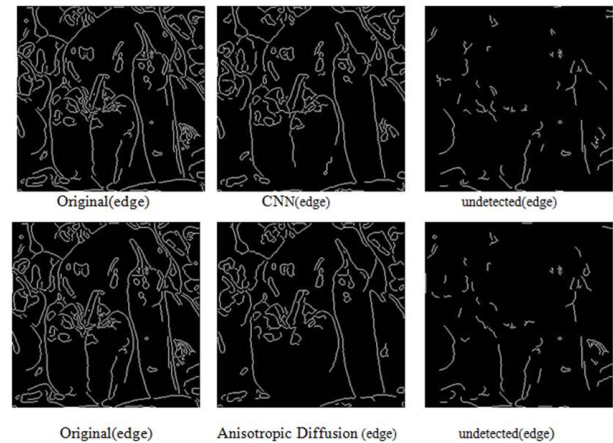
Figure 4(f). The undetected edge comparison between using the Cellular Neural Network and the Anisotropic Diffusion for image denoising (noise type, Speckle and Salt & Pepper)
