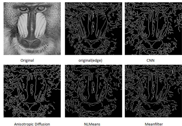
Figure 3(c). The denoising edge protect comparison among the Cellular Neural Network, the Anisotropic Diffusion, the non local means, and the mean filter (noise type, Speckle)
