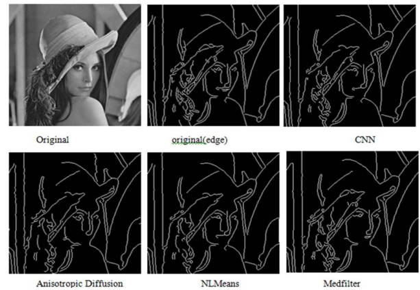
Figure 3(b). The denoising edge protect comparison among the Cellular Neural Network, the Anisotropic Diffusion, the non local means, and the mean filter (noise type, Salt & Pepper)
