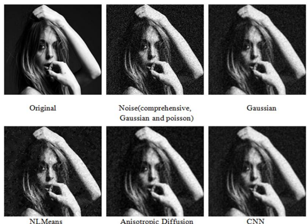
Figure2 (g). The denoising effect comparison among the Gaussian filter, the non local means, the Anisotropic Diffusion, and the Cellular Neural Network
