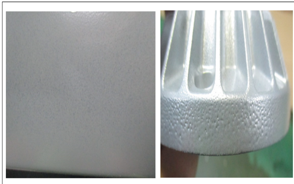
Figure 16 Photos of film thickness defect
