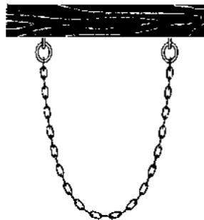
Figure 2: The catenary curve is formed by extending a chain from two fixed points.
