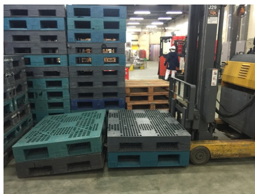
Figure 4-3 Behavior 3: Not using the edge of fork to lift pallet's product
