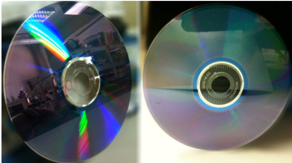
Figure 3.8 Diffraction on DVD plate, from one incident angle (right) and from many (left).
