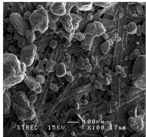
Kraft paper coated with nanoclay 60% w/w
