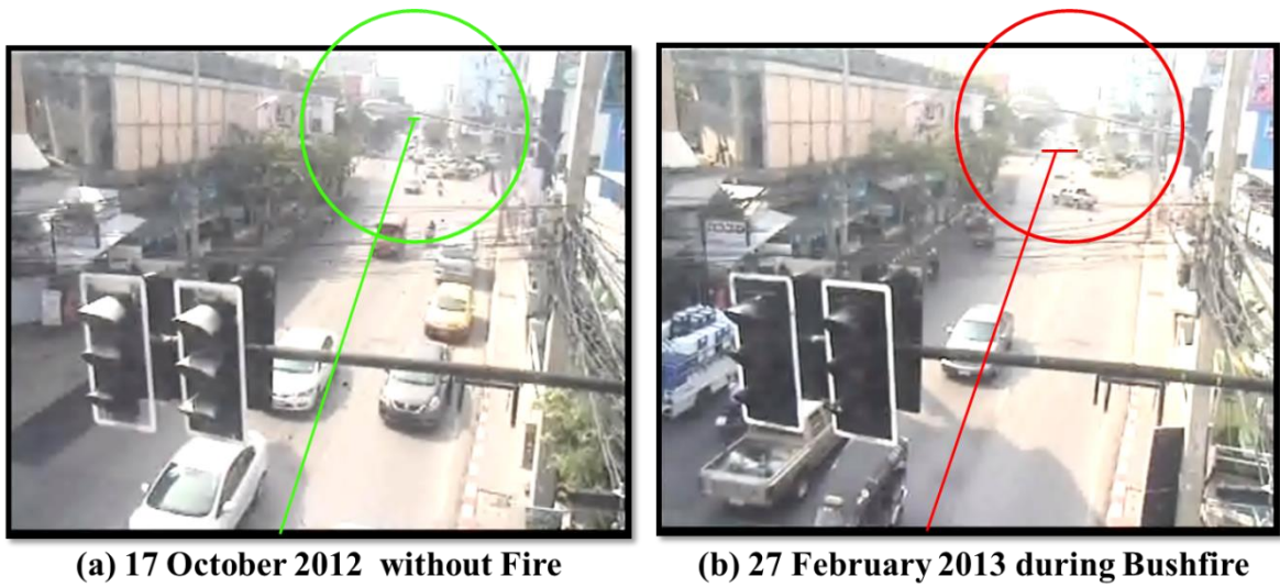
Figure 3: The images from CCTV record from one intersection in Chiang Mai downtown were compared. The visibility lengths, L_v (a) without fire 0.40 m. (b) with fire 0.14 m.
