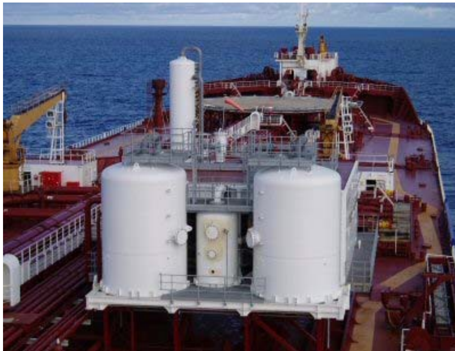
Figure 2.7 Vapor Recovery Systems. (Absorption Carbon Vacuum-Regenerated Adsorption) [6]
