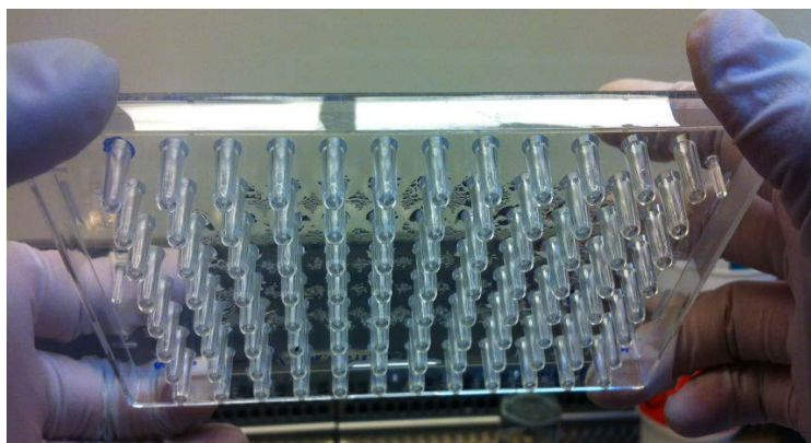
Figure 3.2 Transferable solid phase screening system
