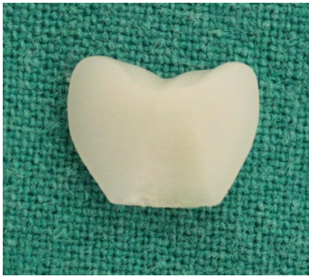
Fig. 4-5: Adhesive failure at framework and veneering interface (Test group A - Fusion with Crystal/Connect)
