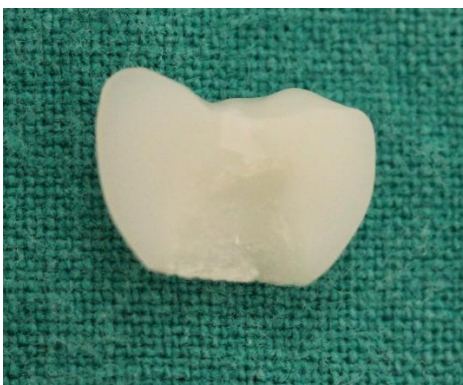
Fig. 4-7: Adhesive failure at framework and veneering interface (Test group B - Bonding with Resin cement)
