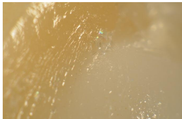
Fig. 4-7: Adhesive failure at framework and veneering interface (Test group B - Bonding with Resin cement)
