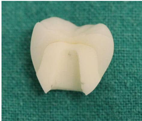
Fig. 4-6: Combination of adhesive and cohesive failure (Test group A - Fusion with Crystal/Connect)
