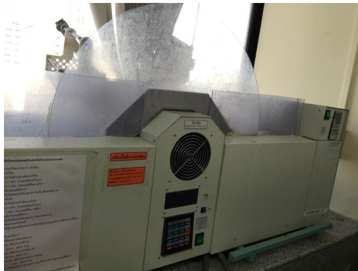
Fig. 3-13: Thermocycling unit (Tc 301, KMIT)
