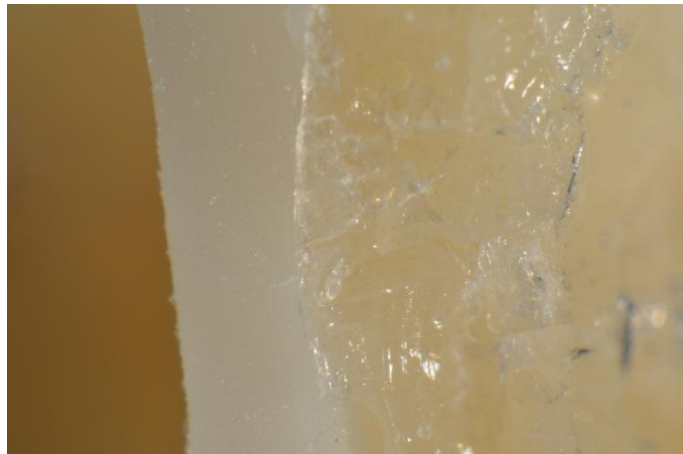
Fig. 4-4: Cohesive failure within veneering layer (Control group - Zirconia based all ceramic)
