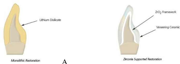
Fig. 2-1: A: Monolithic ceramics. B: Veneering ceramics with framework (Source: R&D Ivoclar Vivadent)
