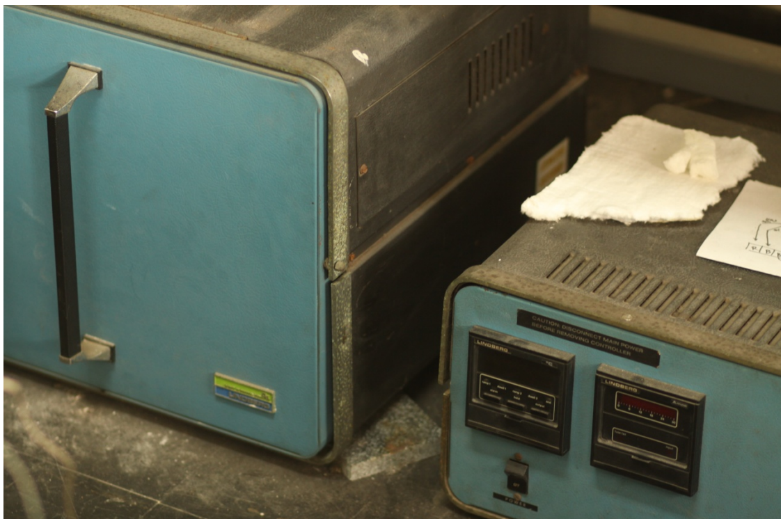
Figure 4.3 Box furnace used to prepare the polycrystalline samples.
