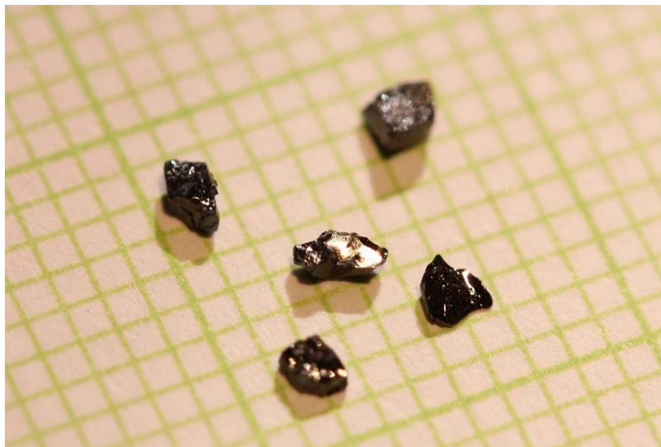
Figure 4.15 Single crystal of \text{BaCu}_2\text{V}_2\text{O}_8 with dimension \sim 1.5\text{mm}^3
