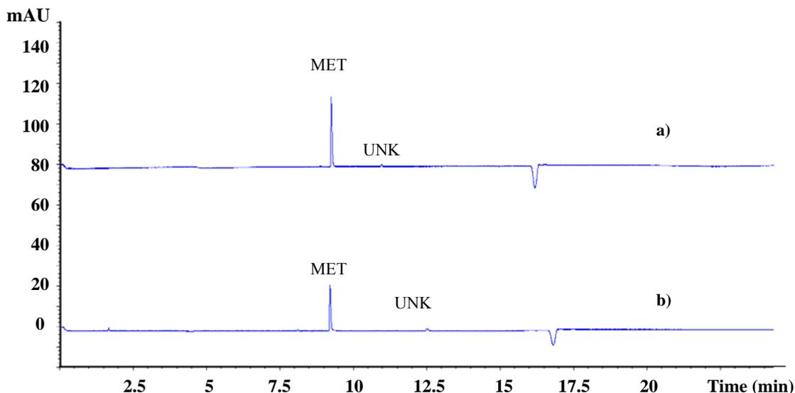
Figure 4.23 Electropherograms of MET degradation exposed to sunlight a) in 0.1N HCl for 30 days, b) in 0.1 N NaOH for 7 days, CE conditions: as Figure 4.6.
