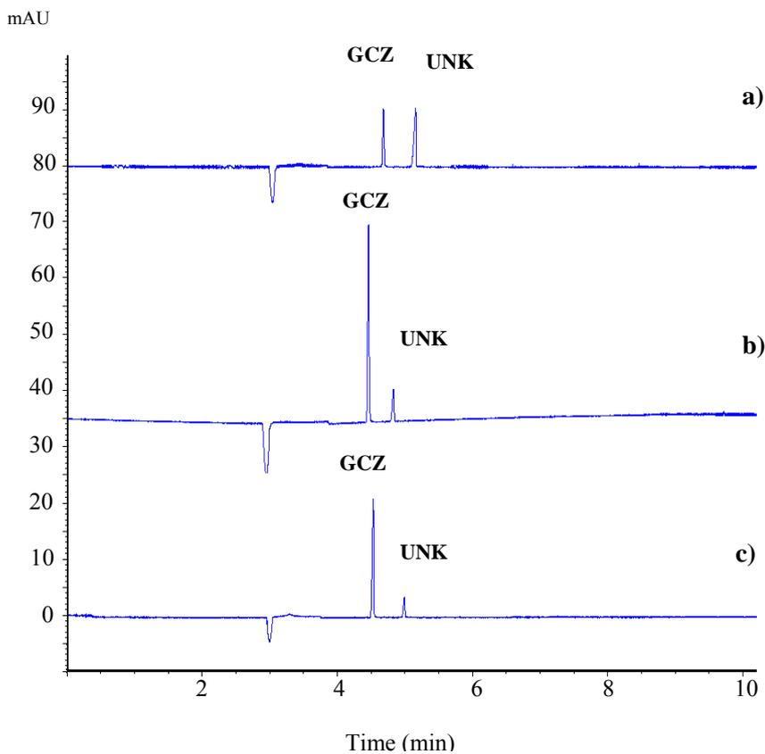
Figure 4.27 Electropherograms of GCZ degradation at 80°C a) in 0.1 N HCl for 10 min, b) in water for 10 min, c) in 3% H<sub>2</sub>O<sub>2</sub> for 10 min. CE conditions: as MEKC method
