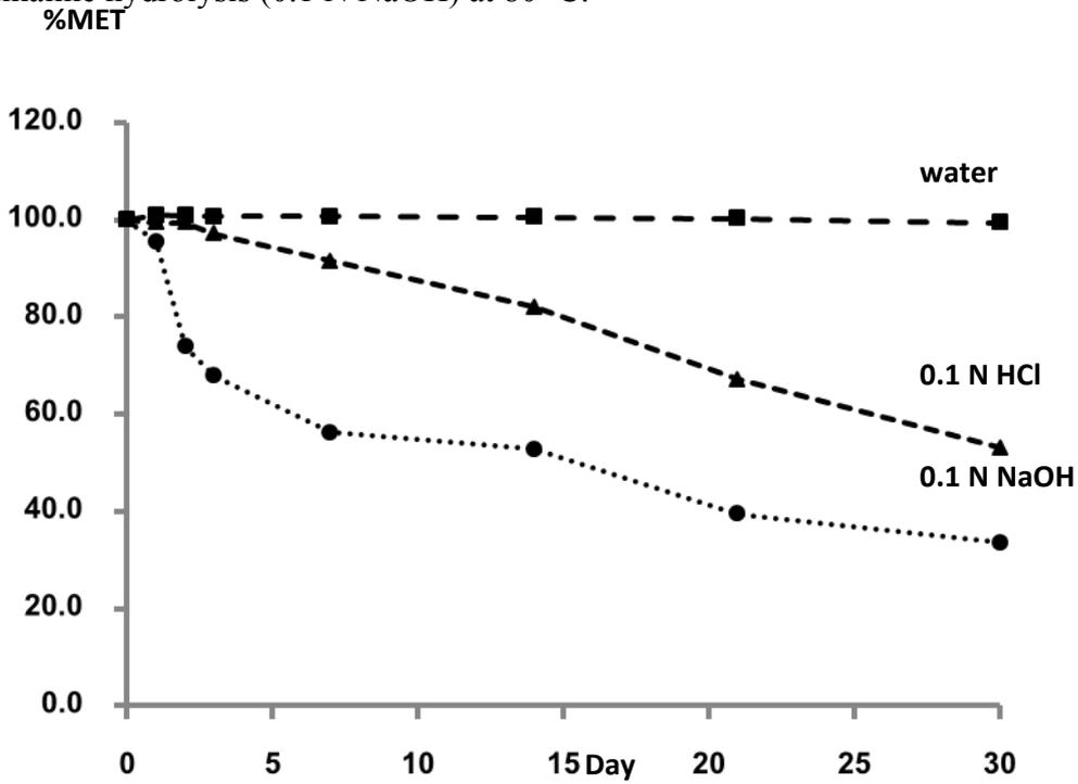
Figure 4.17 Stability profiles for the degradation of MET under neutral (water), acid (0.1 N HCl) and alkaline (0.1 N NaOH) hydrolysis at room temperature (kept in a dark cabinet) (CGN was not observed under these stress conditions).
