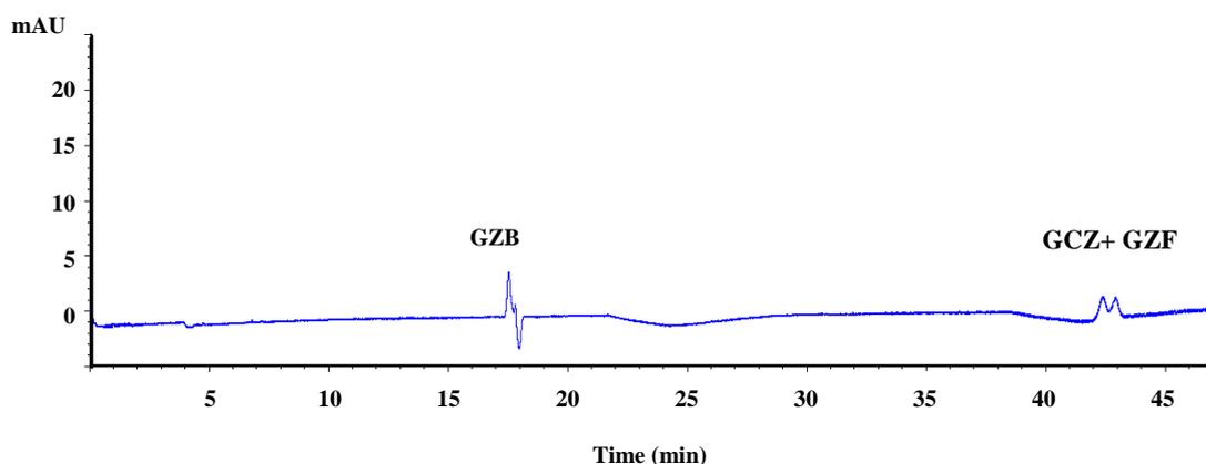
Figure 4.8 Electropherogram on the separation of GCZ (150  $\mu\text{g/mL}$ ), GZB and GZF (200  $\mu\text{g/mL}$ ) Condition: 40mM citrate buffer pH 6.7 ; capillary 68.5cm full length, 60 cm effective length, 50 $\mu\text{m}$  ID, injection at 50 mbar, 5 s; 15 kV; 30  $^{\circ}\text{C}$ ; detection by DAD absorbance at 225 nm.
