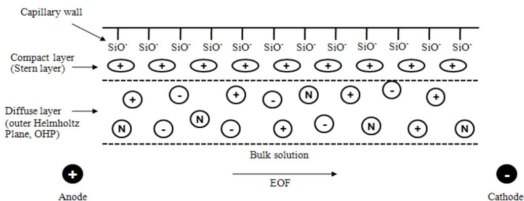
Figure 2.5 Electrical double layer at the ionized silica capillary wall and illustration of EOF (60)
