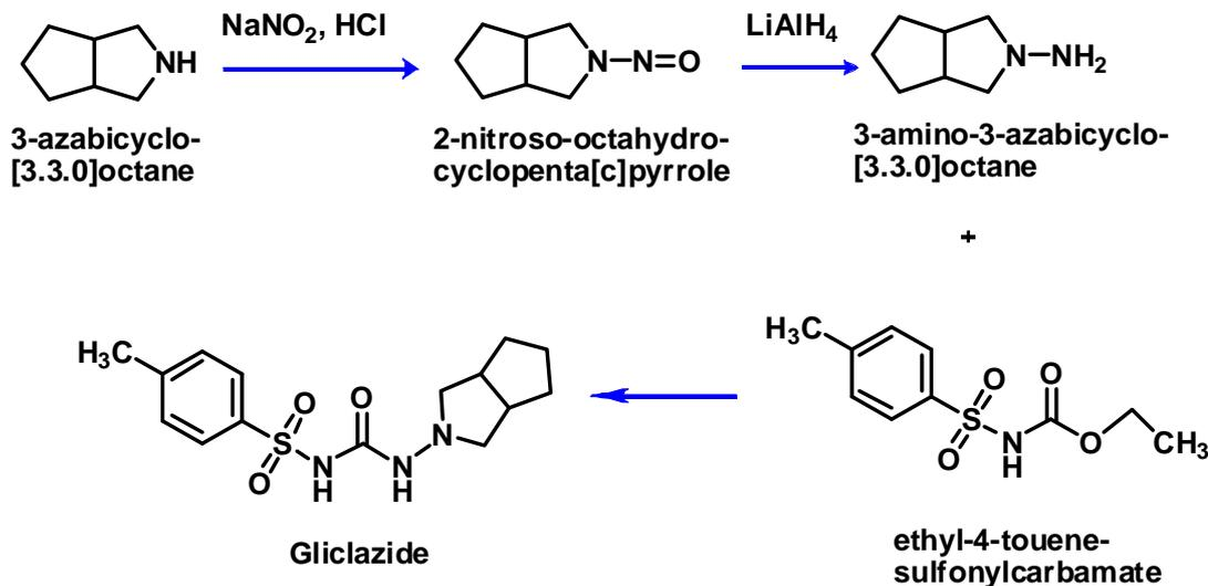
Figure 2.3 Synthesis of gliclazide
