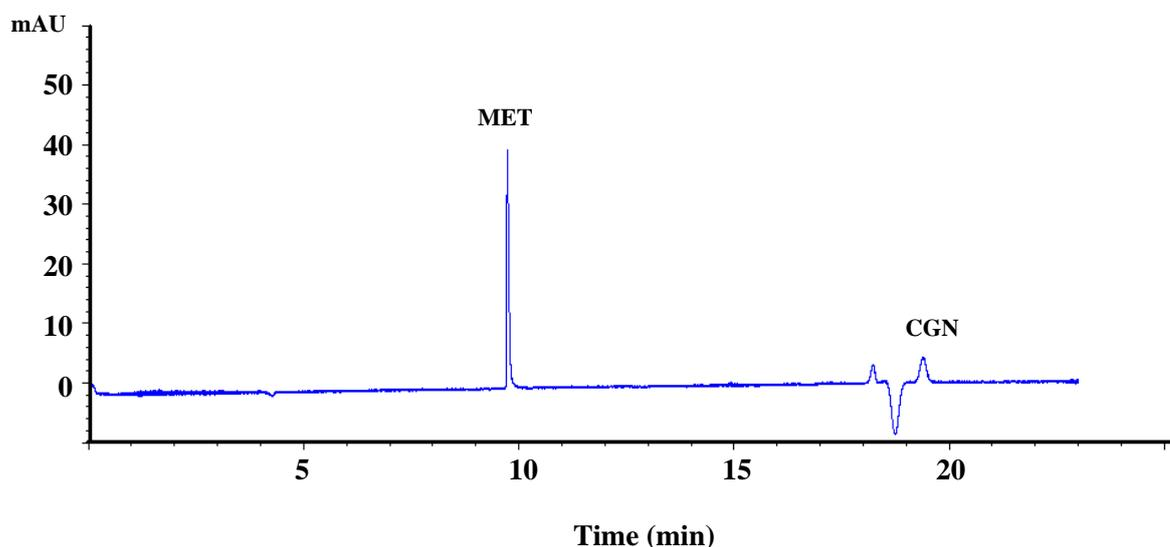
Figure 4.7 Electropherogram of the optimum condition on the separation of MET (600  $\mu\text{g}/\text{mL}$ ) and CGN (40  $\mu\text{g}/\text{mL}$ ). Condition: BGE: 40 mM citrate buffer pH 6.7 ; capillary 68.5cm full length, 60 cm effective length, 50 $\mu\text{m}$  ID, injection at 50 mbar, 5 s; voltage 15 kV; temperature 30  $^{\circ}\text{C}$ ; detection by DAD absorbance at 214 nm.
