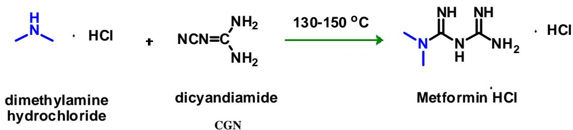
Figure 2.2 Synthesis of metformin.
