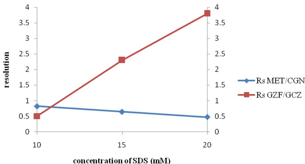
Figure 4.10 Plot of concentration of SDS vs. resolution of MET/CGN and resolution of GZF/GCZ. Conditions: BGE: various concentration of SDS (10, 15 and 20 mM) in 10 mM sodium dihydrogen phosphate buffer pH 7.0; capillary 64.5cm full length, 56 cm effective length, 50 $\mu$ m ID, injection at 50 mbar, 5 s; voltage 20 kV; temperature 25  $^{\circ}$ C; detection by DAD absorbance at 225 nm.
