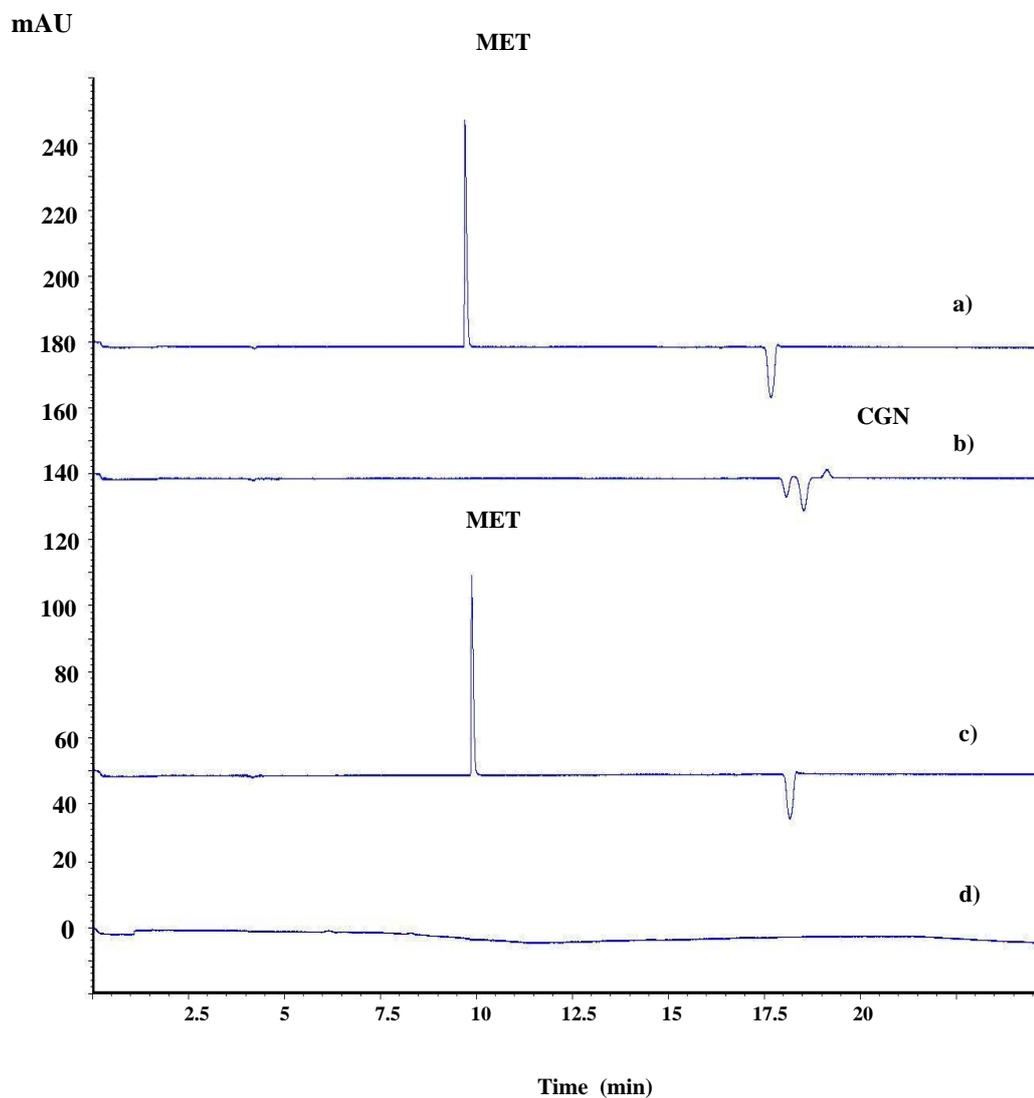
Figure 4.13 Electrochromatogram of a) standard MET (500  $\mu\text{g/mL}$ ), b) standard CGN (10  $\mu\text{g/mL}$ ), c) sample MET (500  $\mu\text{g/mL}$ ), d) BGE; BGE Condition: 40 mM citrate buffer pH 6.7 ; capillary 68.5cm full length, 60 cm effective length, 50 $\mu\text{m}$  ID, injection at 50 mbar, 5 s; voltage 15 kV; temperature 30°C; detection by DAD absorbance at 214 nm.
