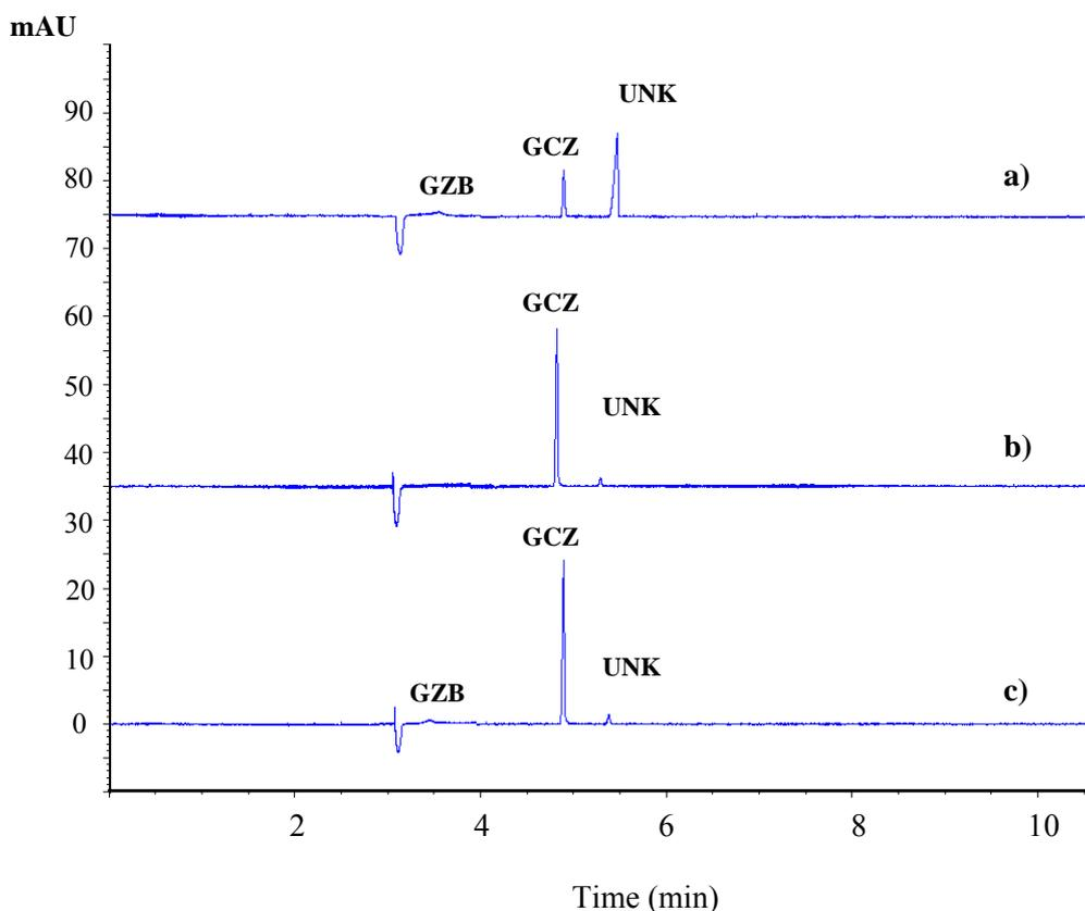
Figure 4.28 Electropherograms of GCZ degradation at room temperature (kept in a dark cabinet, after 3 days) a) in 0.1 N HCl, b) in water and c) in 3% H<sub>2</sub>O<sub>2</sub>. CE conditions: as MEKC method
