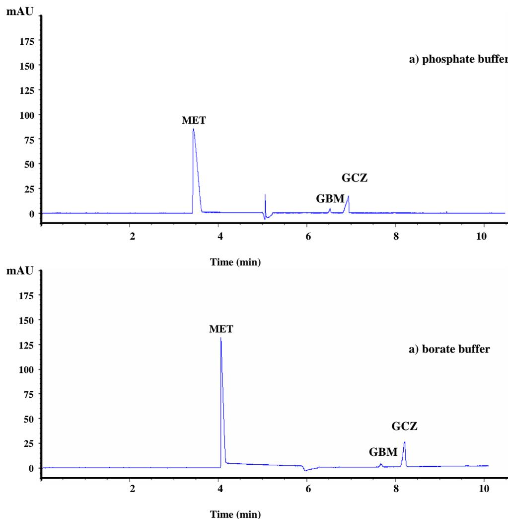
Figure 4.2 Effects of types of buffer on the separation of MET, GBM and GCZ (concentration 1,000  $\mu\text{g/mL}$ , 10  $\mu\text{g/mL}$ , 100  $\mu\text{g/mL}$ , respectively). Condition: BGE: a) 10 mM sodium dihydrogen phosphate pH 7.0 and b) 50 mM borate buffer pH 9.0; capillary 64.5cm full length, 56 cm effective length, 50 $\mu\text{m}$  ID, injection at 50 mbar, 10 s; temperature 25  $^{\circ}\text{C}$ ; voltage 20 kV; detection by DAD absorbance at 225 nm.
