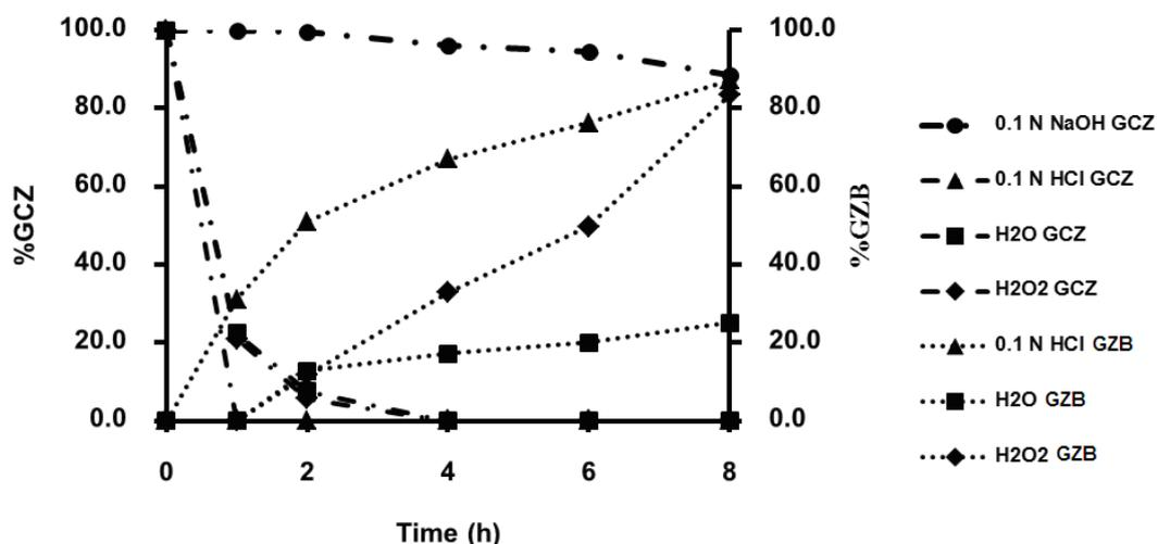
Figure 4.24 Stability profiles for the degradation of GCZ and GZB formation under alkaline (0.1 N NaOH), neutral (water) and acid (0.1 N HCl) hydrolysis and oxidation (3% H<sub>2</sub>O<sub>2</sub>) at 80 °C (GZB was not observed in alkaline hydrolysis).
