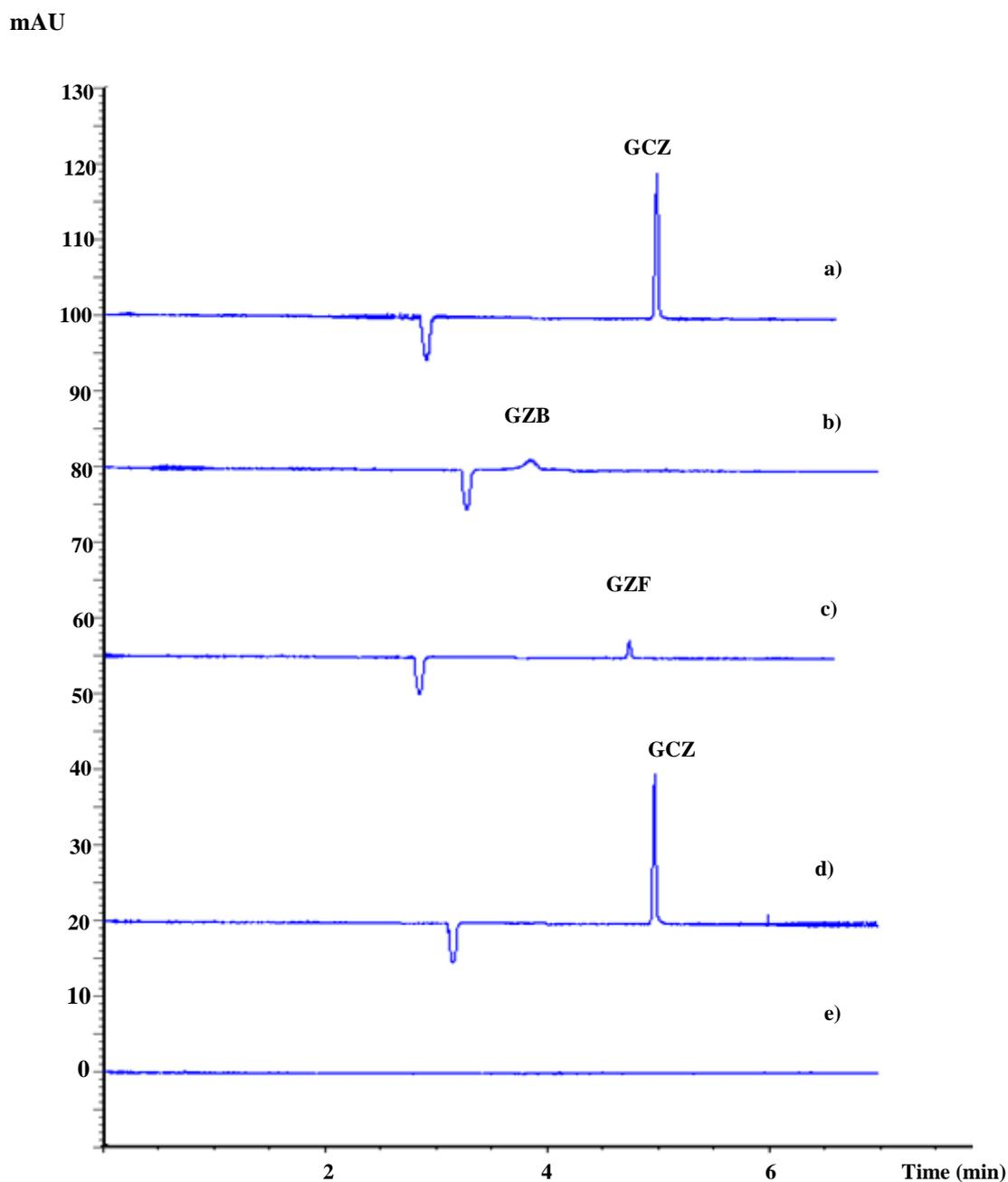
Figure 4.14 Electrochromatogram of a) BGE, b) sample GCZ (160  $\mu\text{g/mL}$ ), c) standard GZF (30  $\mu\text{g/mL}$ ), d) standard GZB (40  $\mu\text{g/mL}$ ), e) standard GCZ (160  $\mu\text{g/mL}$ ), Condition: 10 mM sodium dihydrogen phosphate buffer pH 7.0 adding 15 mM SDS ; capillary 48.5cm full length, 40 cm effective length, 50 $\mu\text{m}$  ID, injection at 50 mbar, 5 s; voltage 20 kV; temperature 25  $^{\circ}\text{C}$ ; detection by DAD absorbance at 225 nm.
