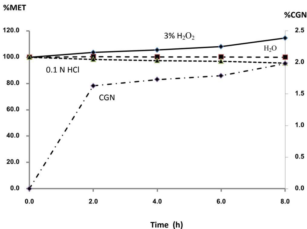
Figure 4.15 Stability profiles for the degradation of MET and CGN formation under neutral (water) and acid (0.1 N HCl) hydrolysis and oxidation (3% H<sub>2</sub>O<sub>2</sub>) at 80 °C (CGN was observed only from oxidation condition)
