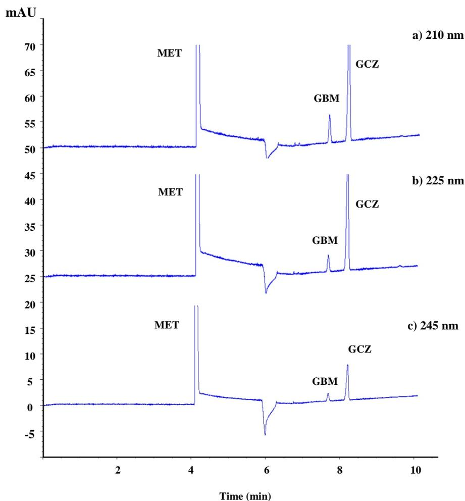
Figure 4.3 Effects of detection wavelength on the separation of MET, GBM and GCZ (concentration 1,000  $\mu\text{g/mL}$ , 10  $\mu\text{g/mL}$ , 100  $\mu\text{g/mL}$ , respectively); Condition: BGE: 50 mM borate buffer pH 9.0; capillary 64.5 cm full length, 56 cm effective length, 50  $\mu\text{m}$  ID, injection at 50 mbar, 10 s; temperature 25  $^{\circ}\text{C}$ ; voltage 20 kV; varied detection wavelength at a) 210 nm, b) 225 nm, c) 245 nm.
