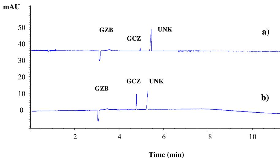
Figure 4.29 Electropherograms of GCZ degradation exposed to sunlight a) in water for 14 days and b) in 0.1 N HCl for 3 days. CE conditions: as MEKC method
