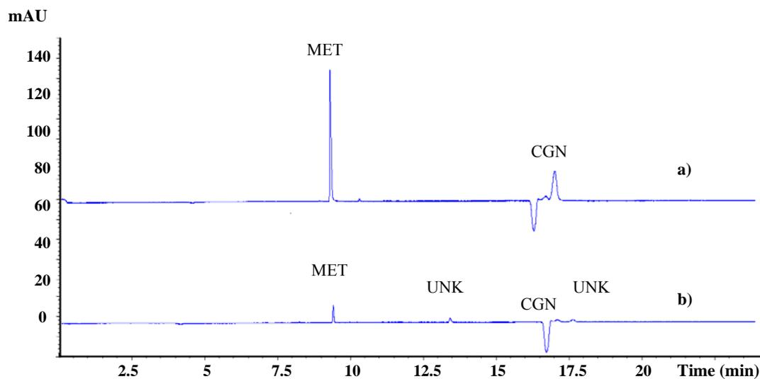
Figure 4.21 Electropherograms of MET degradation under heated at 80°C for 8 h, a) in 3% $H_2O_2$ , b) in 0.1 N NaOH, CE conditions: as Figure 4.6.
