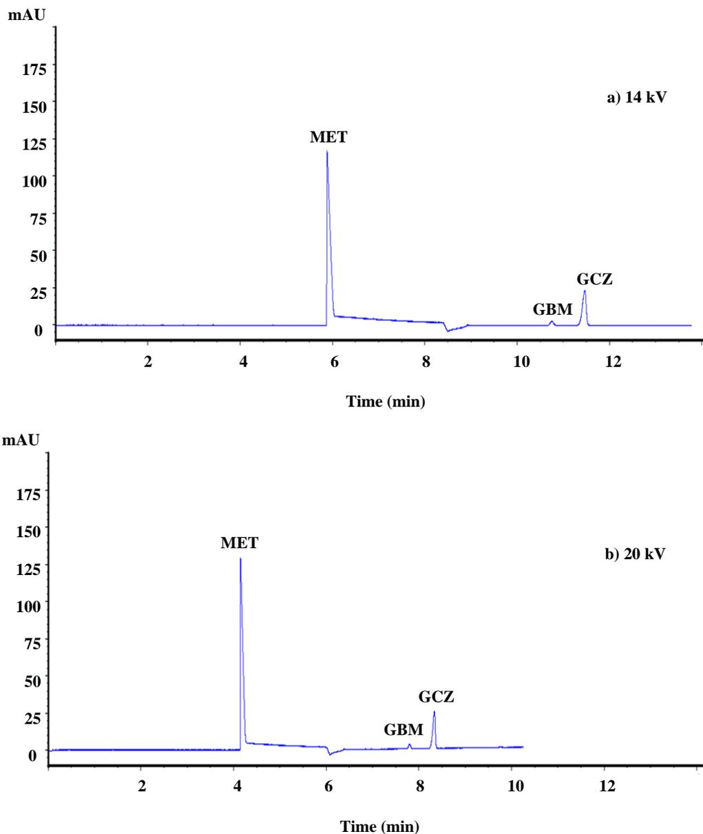
Figure 4.1 Electropherogram of applying voltage effects on the separation of MET, GBM and GCZ (concentration 1,000  $\mu\text{g/mL}$ , 10  $\mu\text{g/mL}$ , 100  $\mu\text{g/mL}$ , respectively). Condition: BGE: 50 mM borate buffer pH 9.0; capillary 64.5cm full length, 56 cm effective length, 50 $\mu\text{m}$  ID, injection at 50 mbar, 10 s; temperature 25  $^{\circ}\text{C}$ ; voltage a) 14 kV and b) 20 kV; detection by DAD absorbance at 225 nm.
