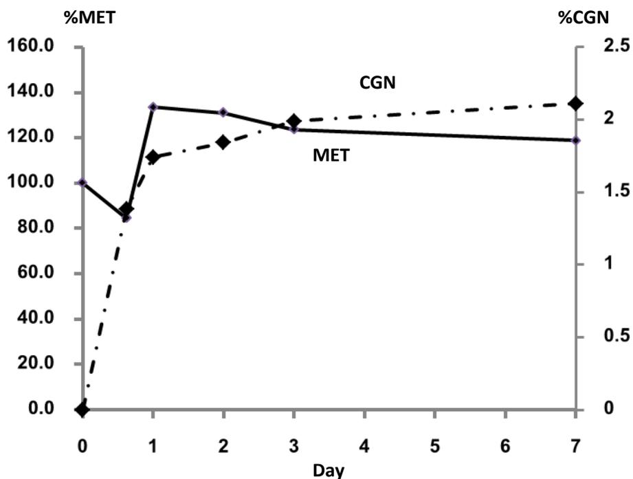
Figure 4.18 Stability profiles for the degradation of MET and CGN formation under oxidation (3% H<sub>2</sub>O<sub>2</sub>) at room temperature (kept in a dark cabinet).
