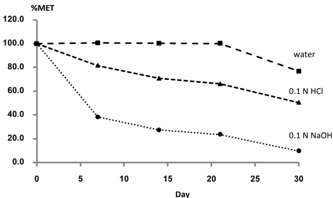
Figure 4.19 Stability profiles for the degradation of MET and CGN formation under neutral (water), acid (0.1 N HCl) and alkaline (0.1 N NaOH) exposed to sunlight.
