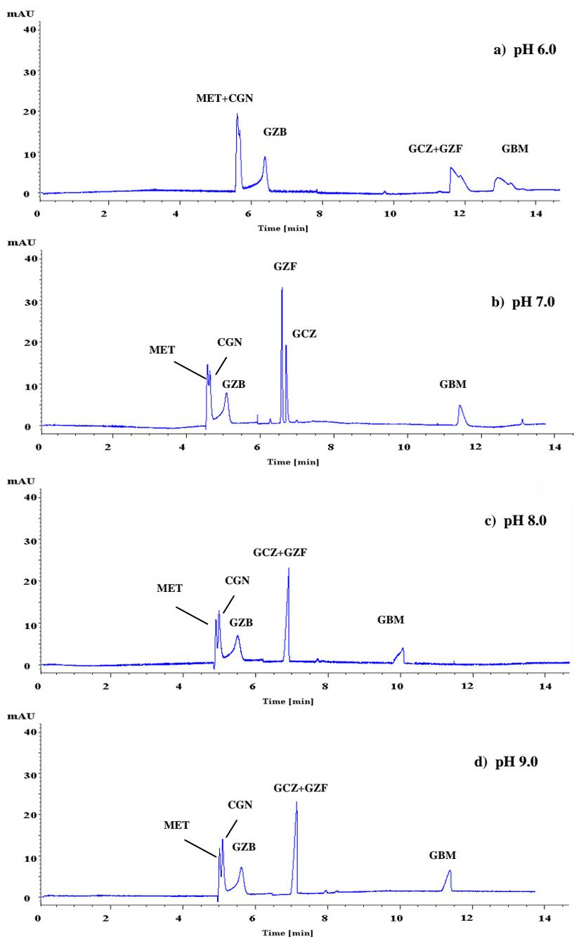
Figure 4.11 Electropherogram of pH effects on the separation of MET,CGN, GBM, GCZ (100 $\mu$ g/mL), GZB,GZF (200 $\mu$ g/mL) Condition: 10 mM sodium dihydrogen phosphate buffer containing 15 mM SDS with varied pH: a) pH 6.0, b) pH 7.0, c) pH 8.0, d) pH 9.0 ; capillary 64.5cm full length, 50 cm effective length, 50 $\mu$ m ID, injection at 50 mbar, 5 s; 20 kV; 25 °C; detection by DAD absorbance at 225 nm.
