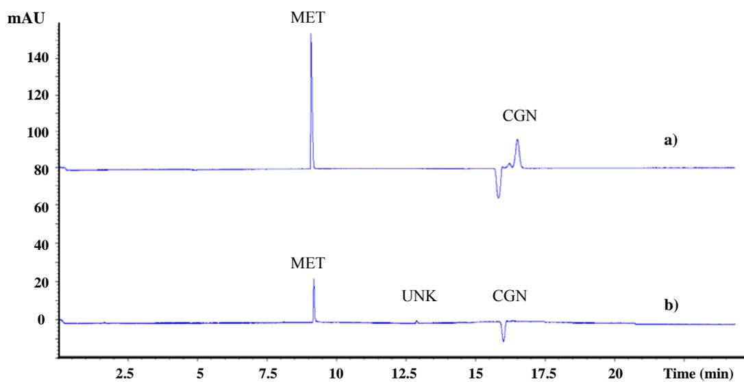
Figure 4.22 Electropherograms of MET degradation at room temperature (kept in a dark cabinet), a) in 3% $H_2O_2$  for 1 day, b) in 0.1 N NaOH for 30 days, CE conditions: as Figure 4.6.
