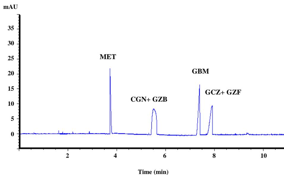
Figure 4.9 Electropherogram of the separation of MET, CGN, GCZ(100 $\mu$ g/mL), GBM, GZB and GZF (200 $\mu$ g/mL) Condition: BGE: 10 mM sodium dihydrogen phosphate buffer pH 7.0 ; capillary 64.5cm full length, 56 cm effective length, 50 $\mu$ m ID, injection at 50 mbar, 5 s; voltage 20 kV; temperature 25  $^{\circ}$ C; detection by DAD absorbance at 225 nm.
