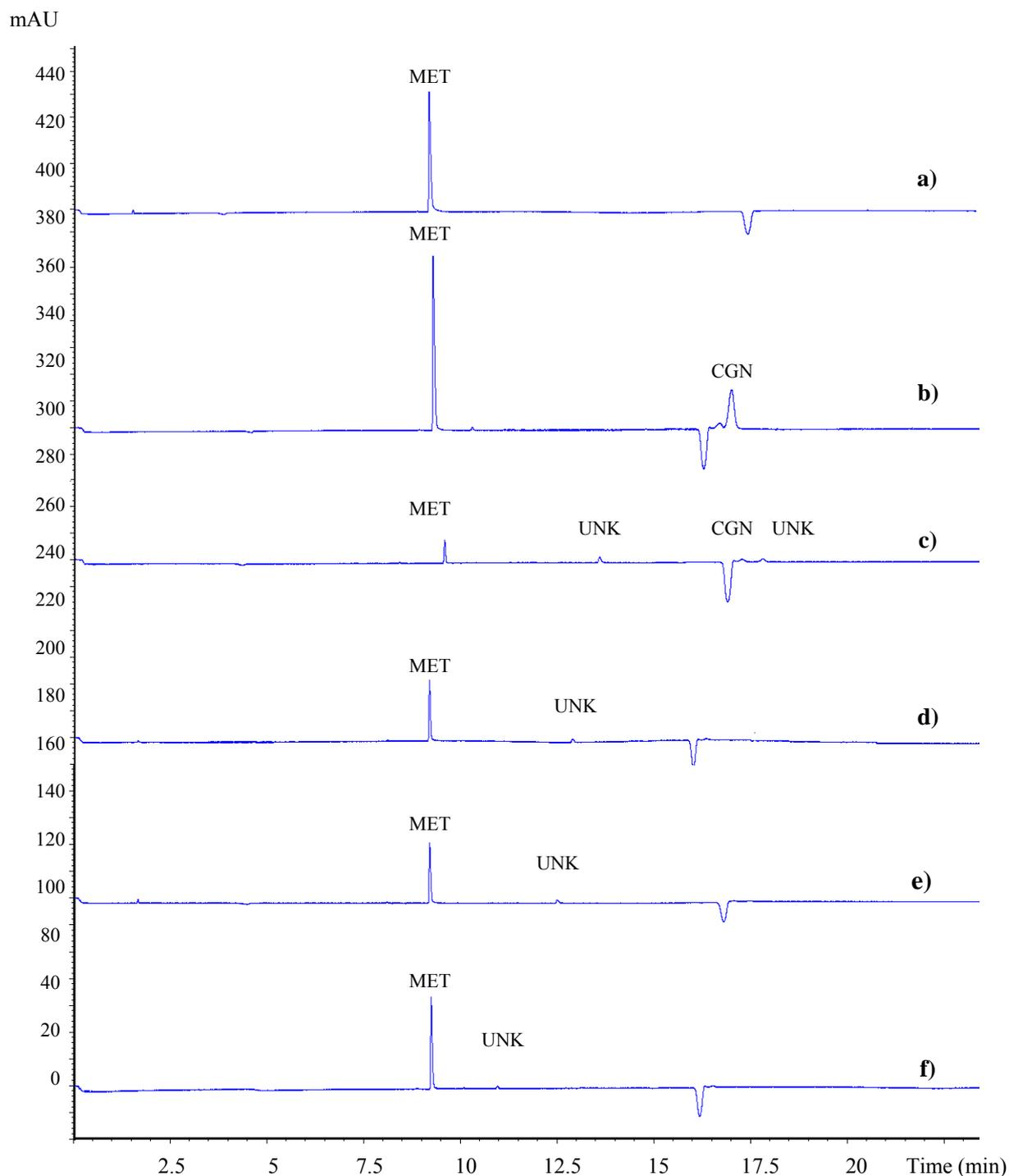
Figure 4.20 Electropherograms of MET degradation under various stress conditions a) Initial, b) in 3% H<sub>2</sub>O<sub>2</sub>, heated at 80°C for 8 h, c) in 0.1 N NaOH, heated at 80°C for 1.5 h d) in 0.1 N NaOH, at room temperature (kept in a dark cabinet for 30 days), e) in 0.1 N NaOH, exposed to sunlight for 7 days, f) in 0.1 HCl, exposed to sunlight for 30 days. CE conditions: as Figure 4.6.
