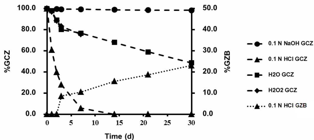
Figure 4.25 Stability profiles for the degradation of GCZ and GZB formation under alkaline (0.1 N NaOH), neutral (water) and acid (0.1 N HCl) hydrolysis and oxidation (3% H<sub>2</sub>O<sub>2</sub>) at room temperature (kept in a dark cabinet) (GZB was observed only in acid hydrolysis).
