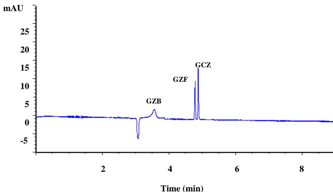
Figure 4.12 MEKC separation of GCZ, GZB and GZF (100 $\mu\text{g}/\text{mL}$ ) Condition : 10 mM sodium dihydrogen phosphate buffer pH 7.0 adding 15 mM SDS ; capillary 48.5cm full length, 40 cm effective length, 50 $\mu\text{m}$  ID, injection at 50 mbar, 5 s; voltage 20 kV; temperature 25  $^{\circ}\text{C}$ ; detection by DAD absorbance at 225 nm.
