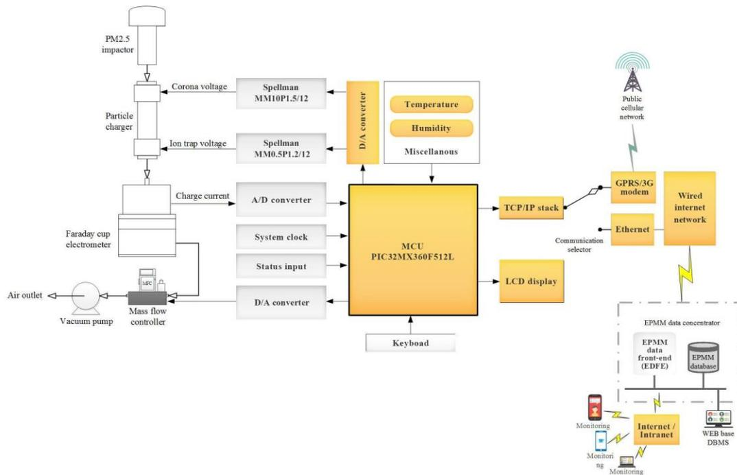
Figure 1. Schematic diagram of the EPMM.
