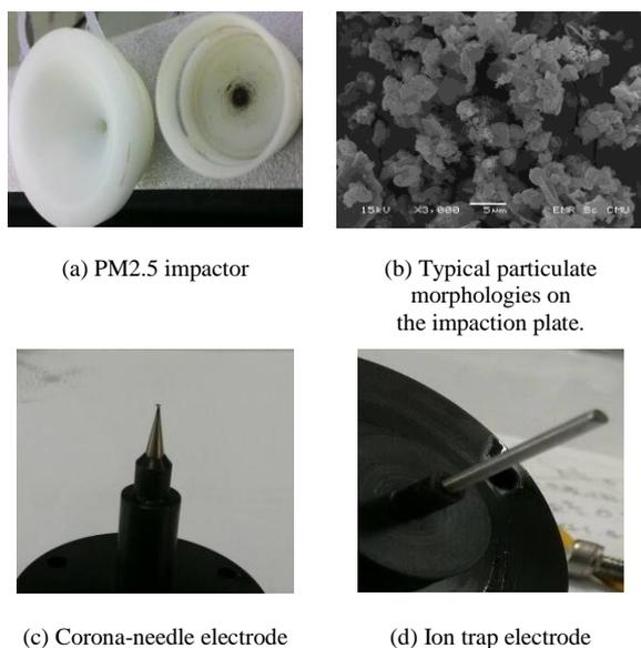
Figure 7. Particulate deposition inside the PM2.5 impactor and particle charger for measuring time of about 507 hour or 21 days.
