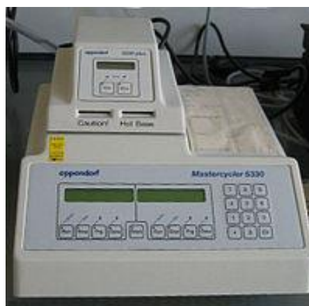
Figure 9 A thermal cycler for PCR.
