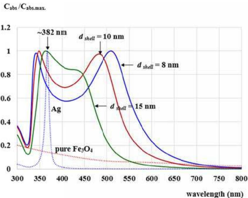
**Figure 5.** Calculated absorption spectra of  $\text{Fe}_3\text{O}_4$ @Ag composite particle with fixed  $\text{Fe}_3\text{O}_4$  core radius ( $R_{core}$ ) of 16 nm. The Ag shell thickness ( $d_{shell}$ ) was varied from 8 nm to 15 nm.
