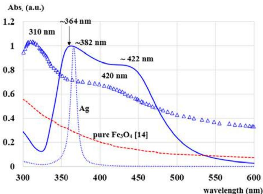
**Figure 2.** Calculated absorption spectra of  $Fe_3O_4$  @Ag composite particle (solid line) compared with two experimental spectra (adapted from Sun *et al.*, 2012) and Ag nanoparticle with particle size of 10 nm. Experimental spectra consist of spectra of pure  $Fe_3O_4$  (dash line) and  $Fe_3O_4$  @Ag core-shell spectra obtained from reaction times of 1 hour (triangle line).
