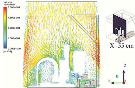
**Figure.7** Velocity vectors in a given yz plane at x=55 cm
