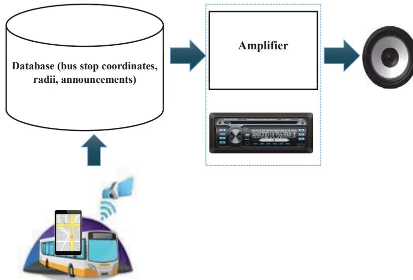
**Figure 2:** Components of the Automatic Announcement System for Public Buses Using a Tablet
