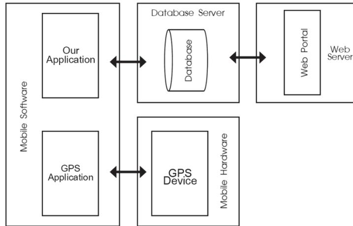
**Figure 4:** A Model of the Android Application for Automatic Announcements on Public Buses
