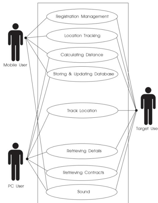
**Figure 5:** The Operation Process of the Use Case Diagram of the Android Application for Automatic Announcements on Public Buses
