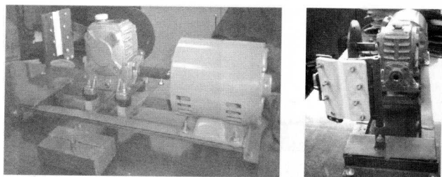
Figure 8 Schematics of plastic pinless butt hinge testing machine
