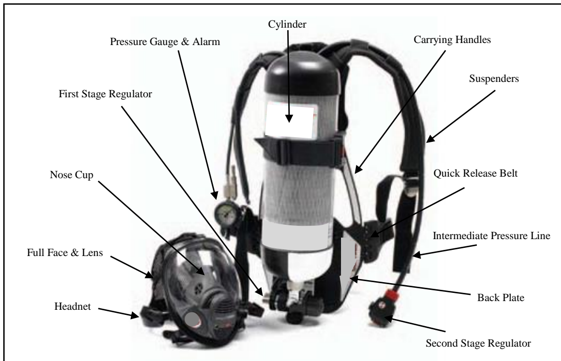
Figure 2.3 Components of the SCBA
