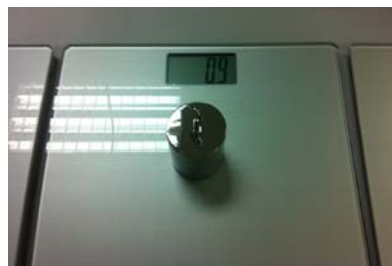
Figure 3.2: Calibration weight scales by the standard weight.
