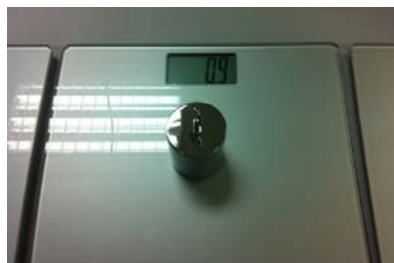
Figure 3.7: Calibration weight scales by the standard weight.
