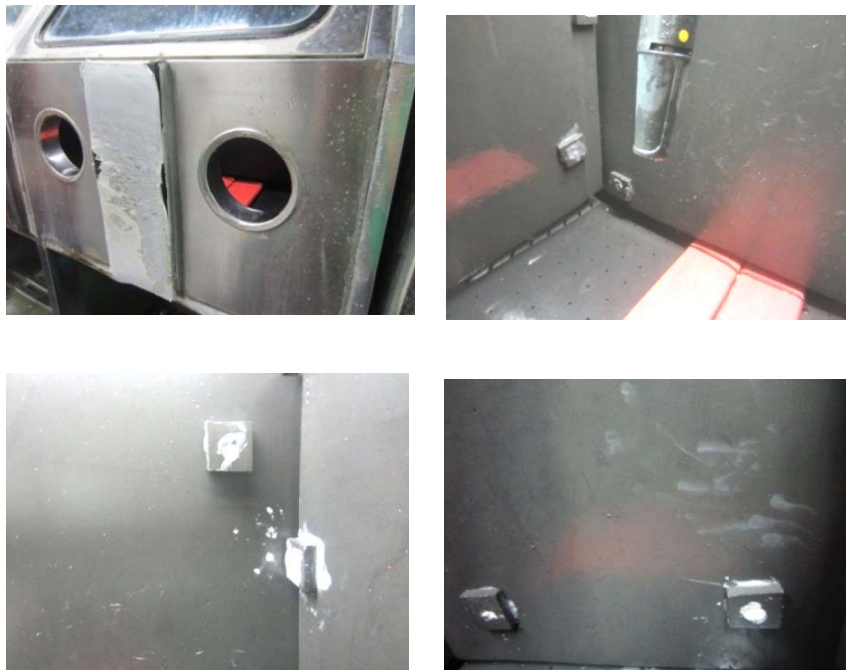
Figure B-6 Installation absorber material inside of Jewelry cleaning machine.
