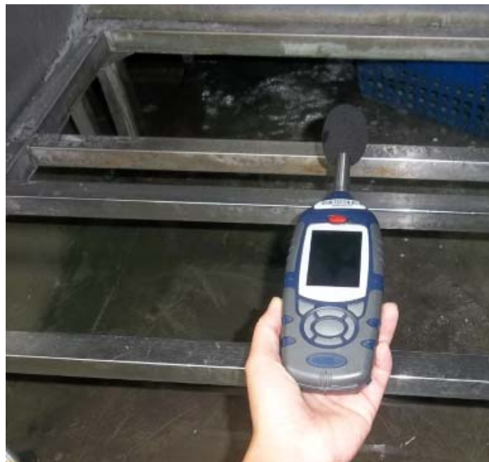
Figure B-14 Noise Monitor at right of the middle of Jewelry cleaning machine
