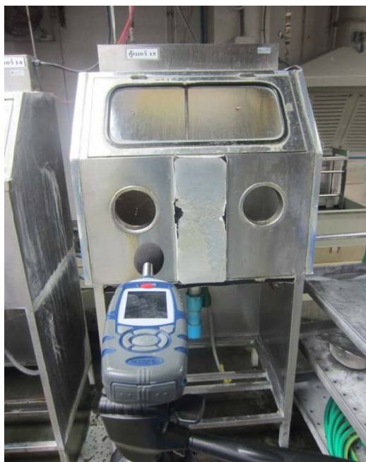
Figure B-8 Noise monitor at lift of the middle of jewelry cleaning machine
