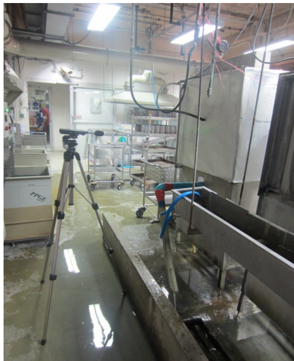
Figure B-12 Noise Monitor at back of the middle of Jewelry cleaning machine
