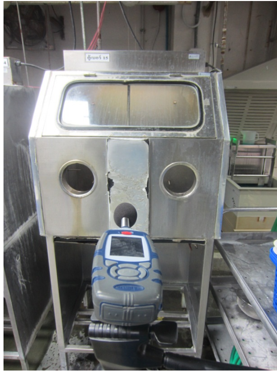
Figure B-9 Noise monitor at middle of Jewelry Cleaning machine
