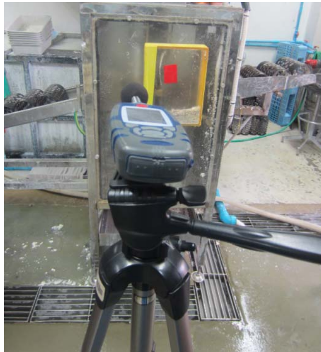
Figure B-3 Noise monitoring at Cleaning box machine.
