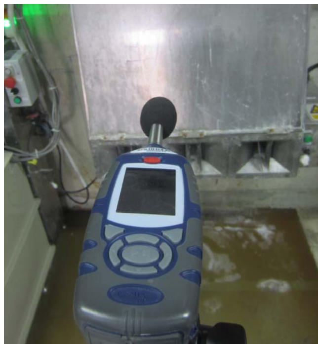
Figure B-4 Noise monitoring at cleaning machine.
