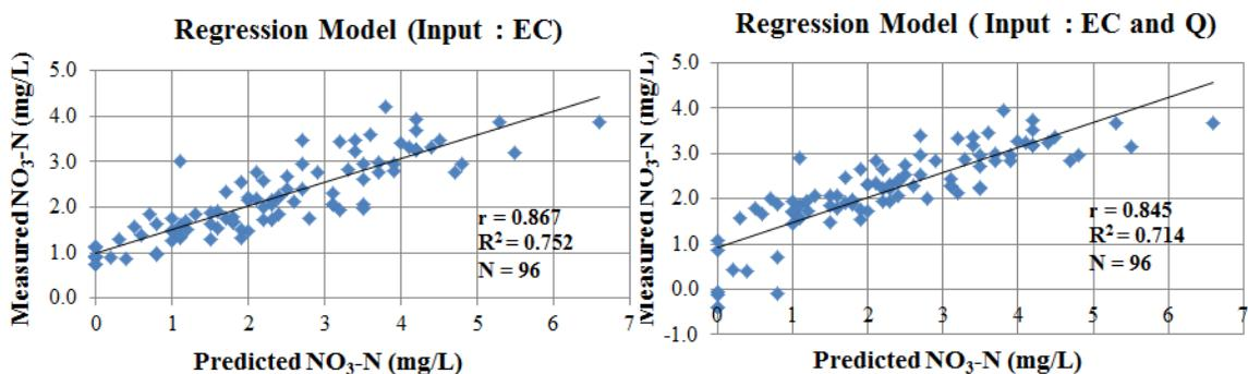
Figure 9. Comparison of the regression model-measured and the predicted NO<sub>3</sub>-N values in U-Tapao canal
