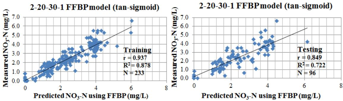
Figure 6. Comparison of the  $\text{NO}_3\text{-N}$  predicted by the FFBP model (with the tan-sigmoid transfer function in the output layer) and the measured  $\text{NO}_3\text{-N}$  in U-Tapao canal
