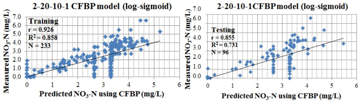
Figure 8. Comparison of the NO<sub>3</sub>-N predicted by the CFBP model (with the log-sigmoid transfer function in the output layer) and measured NO<sub>3</sub>-N values in U-Tapao canal
