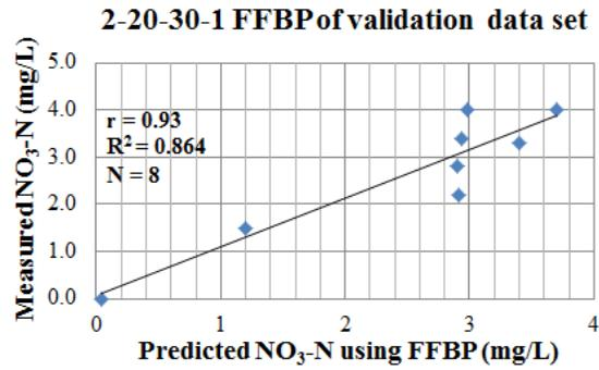
Figure 10. Comparison of the NO<sub>3</sub>-N predicted by the 2-20-30-1 structure FFBP model and the measured values based on the validation data set (n = 8 samples)
