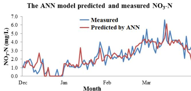
Figure 11. Comparison of ANN model-measured and predicted NO<sub>3</sub>-N values in U-Tapao canal
