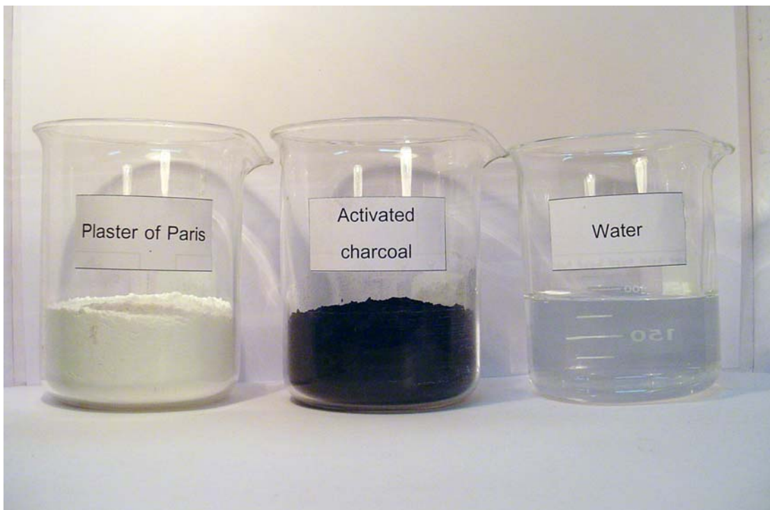
Figure 3-3 Ingredients of plaster of Paris-charcoal substrate
