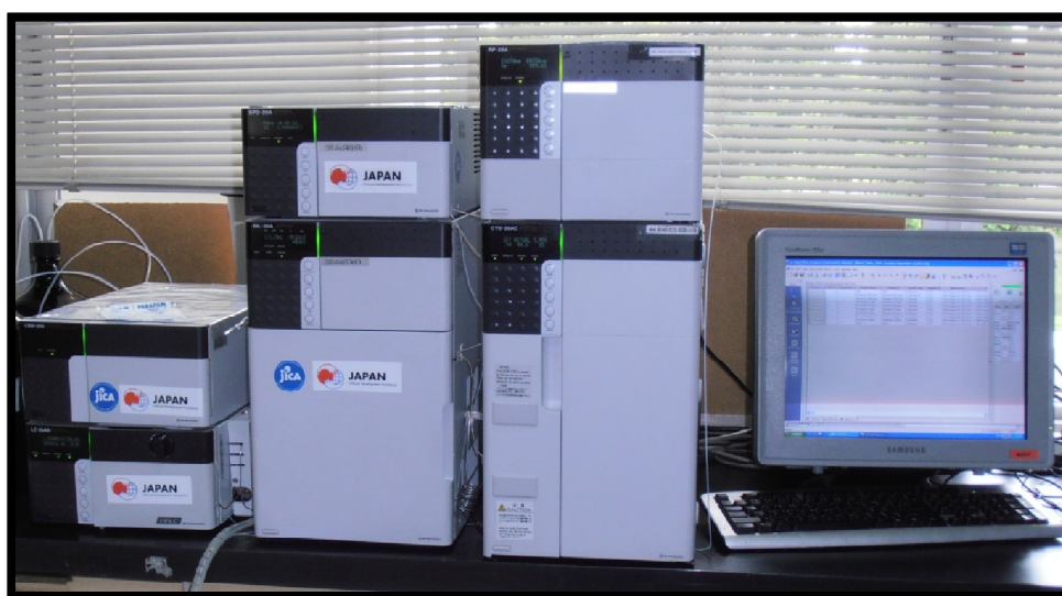
Figure 3.4 High Performance Liquid Chromatography (HPLC) equipped with UV/Vis detector and fluorescence detector, Shimadzu, Japan
