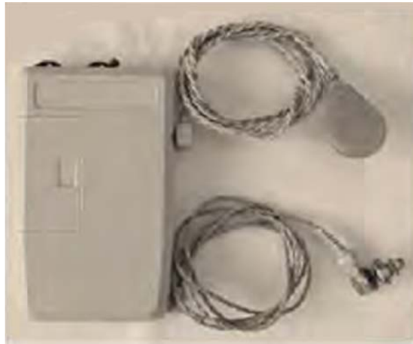
Figure 2.5 The House 3M single channel cochlear implant: the body worn speech processor unit with transmitting coil and microphone cable[42].
