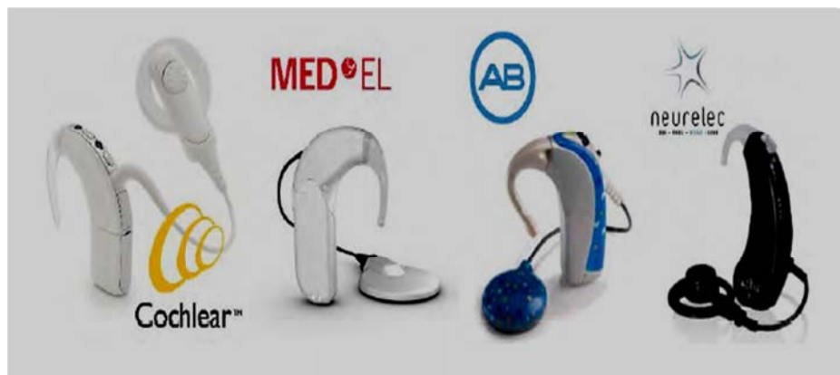
Figure 2.6 The speech processors of the 4 cochlear implant manufacturers: from left to right: Cochlear Ltd., Med-EL Hearing Technologies, Advanced Bionics Corporation and Neurelec [42].
