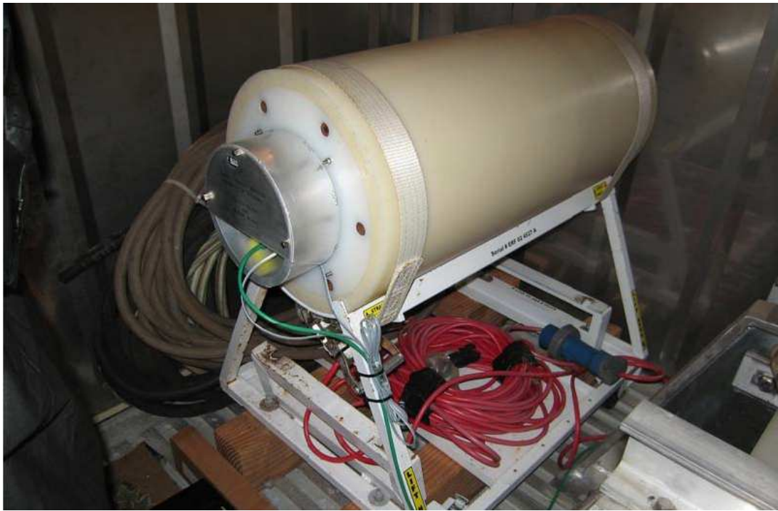
Figure 2.11: Calibration neutron monitor with electronics head from Bartol Research Institute, U. Delaware, USA
