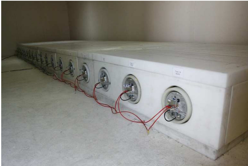
Figure 2.6: The placement of the Princess Sirindhorn Neutron Monitor (an 18NM64 monitor) at Doi Inthanon, Chiang Mai, Thailand
