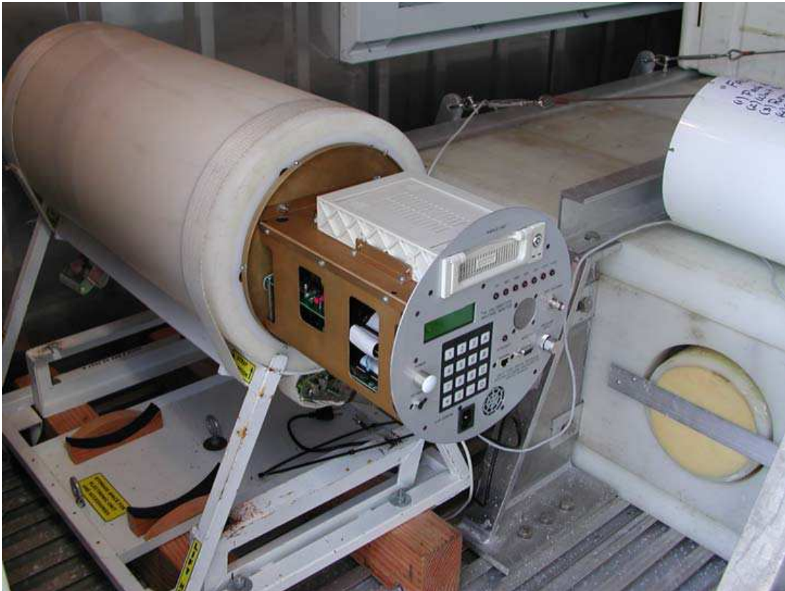
Figure 2.10: Calibration neutron monitor with electronics head (cover removed) from Northwest University, Potchefstroom, South Africa
