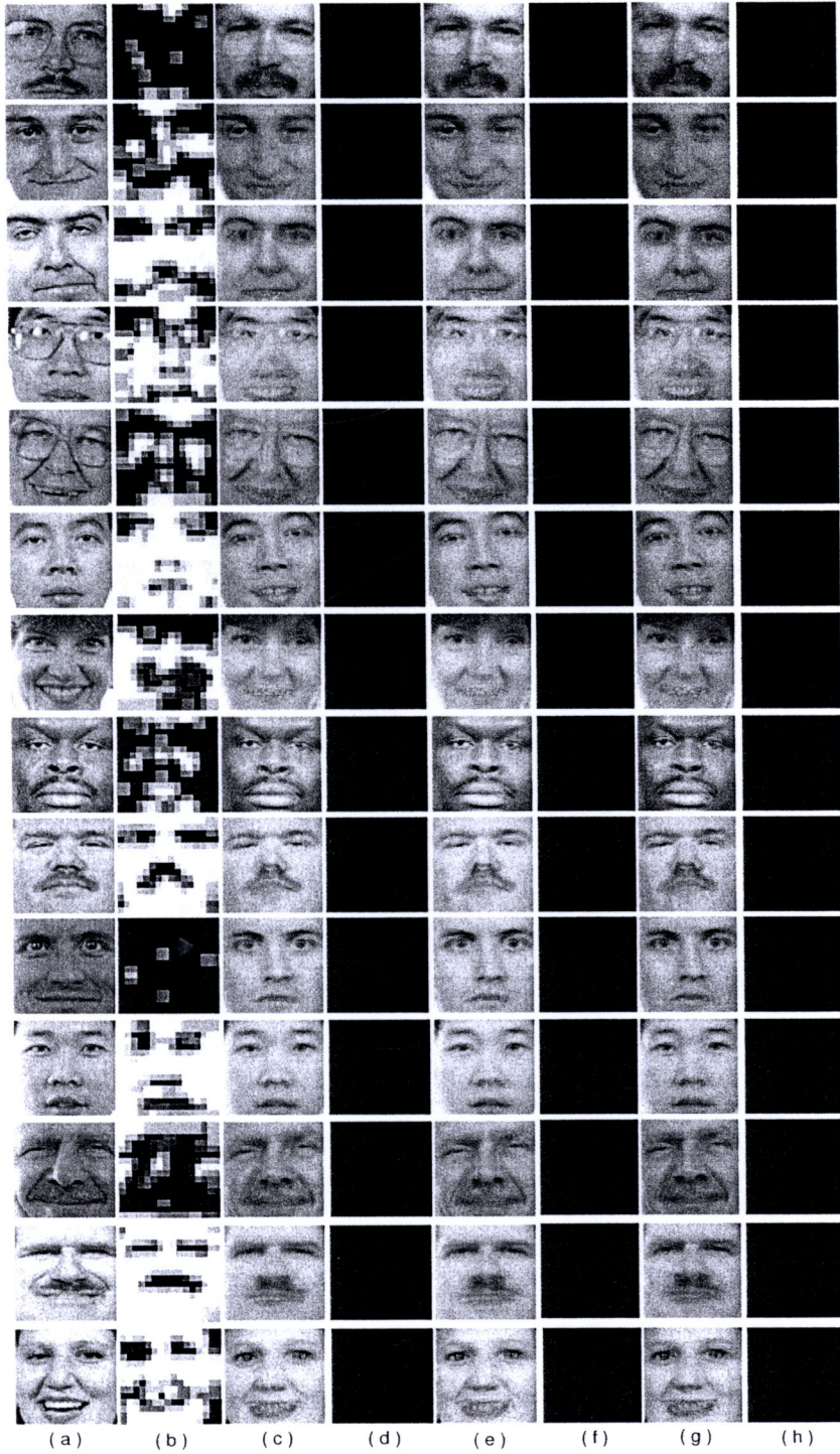
Figure 4: Some of experimental results (HSV color model) with a linear regression model in MPCA method. (a) original HR images ( 30 \times 30 ); (b) input LR images ( 15 \times 15 ) with noise, motion and blur in LR images; (c) face hallucination result with 90 percent MPCA; (d) different image of face hallucination result with 90 percent MPCA; (e) face hallucination result with 95 percent MPCA; (f) different image of face hallucination result with 95 percent MPCA; (g) face hallucination result with 100 percent MPCA; (h) different image of face hallucination result with 100 percent MPCA;
