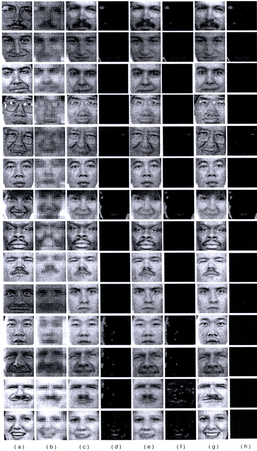
Figure 6: Some of experimental results (RGB color model) with a linear regression model in tensorPCA method. (a) original HR images ( 30 \times 30 ); (b) input LR images ( 15 \times 15 ) with noise, motion and blur in LR images; (c) face hallucination result with 90 percent tensorPCA; (d) different image of face hallucination result with 90 percent tensorPCA; (e) face hallucination result with 95 percent tensorPCA; (f) different image of face hallucination result with 95 percent tensorPCA; (g) face hallucination result with 100 percent tensorPCA; (h) different image of face hallucination result with 100 percent tensorPCA;
