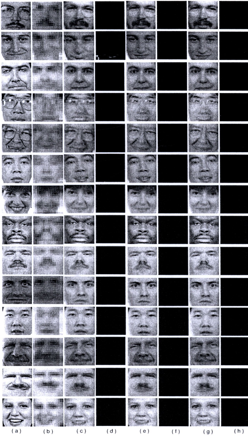
Figure 7: Some of experimental results (YCbCr color model) with a linear regression model in tensorPCA method. (a) original HR images ( 30 \times 30 ); (b) input LR images ( 15 \times 15 ) with noise, motion and blur in LR images; (c) face hallucination result with 90 percent tensorPCA; (d) different image of face hallucination result with 90 percent tensorPCA; (e) face hallucination result with 95 percent tensorPCA; (f) different image of face hallucination result with 95 percent tensorPCA; (g) face hallucination result with 100 percent tensorPCA; (h) different image of face hallucination result with 100 percent tensorPCA;
