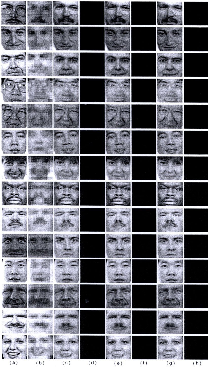
Figure 3: Some of experimental results (YCbCr color model) with a linear regression model in MPCA method. (a) original HR images ( 30 \times 30 ); (b) input LR images ( 15 \times 15 ) with noise, motion and blur in LR images; (c) face hallucination result with 90 percent MPCA; (d) different image of face hallucination result with 90 percent MPCA; (e) face hallucination result with 95 percent MPCA; (f) different image of face hallucination result with 95 percent MPCA; (g) face hallucination result with 100 percent MPCA; (h) different image of face hallucination result with 100 percent MPCA;
