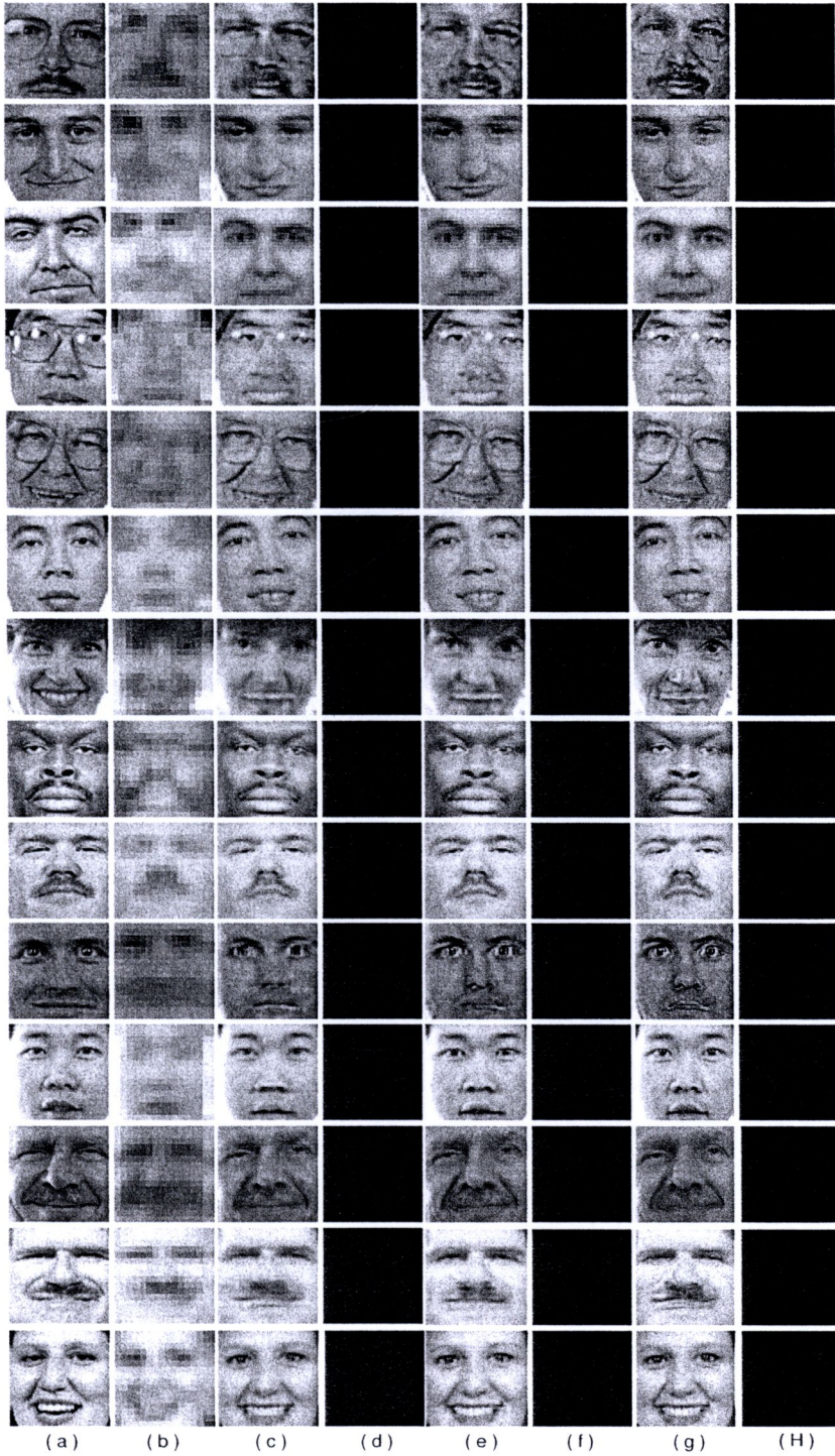
Figure 5: Some of experimental results (CIELAB color model) with a linear regression model in MPCA method. (a) original HR images ( 30 \times 30 ); (b) input LR images ( 15 \times 15 ) with noise, motion and blur in LR images; (c) face hallucination result with 90 percent MPCA; (d) different image of face hallucination result with 90 percent MPCA; (e) face hallucination result with 95 percent MPCA; (f) different image of face hallucination result with 95 percent MPCA; (g) face hallucination result with 100 percent MPCA; (h) different image of face hallucination result with 100 percent MPCA;
