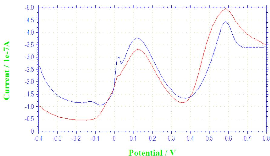
**Figure 4.16** DPV of (GO/PAH/ALP/DI)<sub>1</sub> label drop-dried on SPE towards 0.1 mM PAPP (red) and 0.1 mM PAPP and NADH (blue). Scan rate 20 mV s<sup>-1</sup> and 2 min incubation time.
