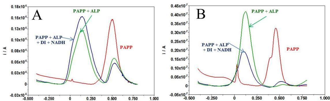
**Figure 4.7** DPV obtained in 0.5 M PBS containing 0.1 M KCl pH 7.0 scan rate 50 mV/s. **A**; 1 mM pAPP (red) 1 mM pAPP with 10 unit of ALP (blue) 1 mM pAPP and 1 mM NADH with 10 unit of ALP and DI (green). **B**; 0.1 mM pAPP (red) 0.1 mM pAPP with 10 unit of ALP (blue) 0.1 mM pAPP and NADH with 10 unit of ALP and DI (green).
