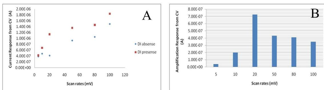
**Figure 4.10** Current response obtained (A) and normalized current (B) at different scan rates using cyclic voltammetry: 5,10, 20, 50, 80, 100 mV/s.
