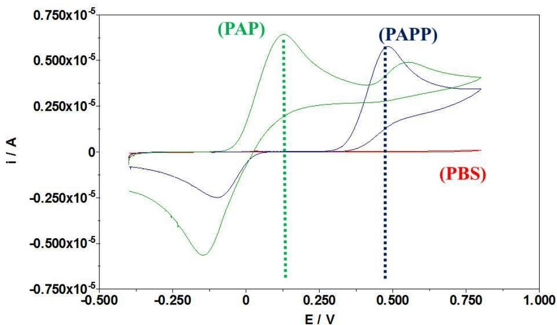
**Figure 4.5** Cyclic voltammograms obtained in 0.1 M PBS containing 0.1 M KCl (pH 8.0) scan rate 50 mV/s. Red line is PBS buffer. Blue line is 1 mM pAPP. Green line is 1 mM pAPP in the presence of Alkaline phosphatase.
