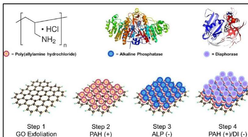
**Figure 4.2** Depiction of layer-by-layer deposition of bi-enzyme on graphene nanoparticles.
