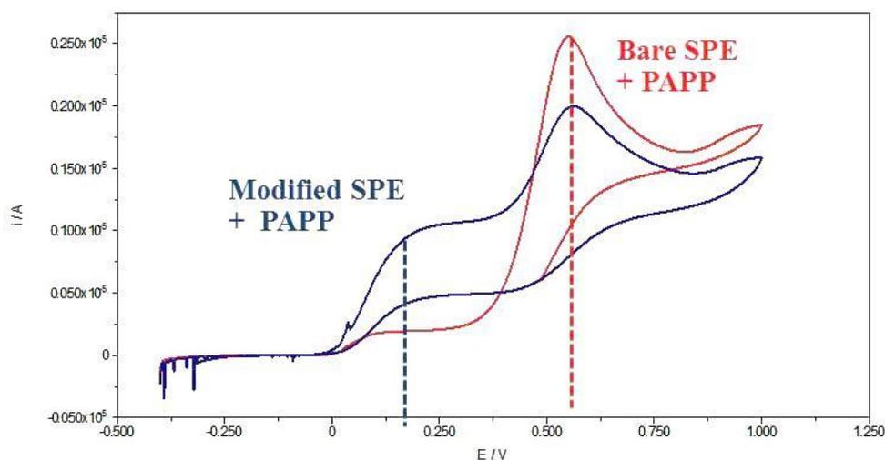
**Figure 4.11** Cyclic voltammograms of bare SPE (red) and modified SPE with GO/PAH/DI layer-by-layer immobilization (blue) toward 2 mM NADH and 0.952 mM PAP. Scan rates 2.5 mV/s.
