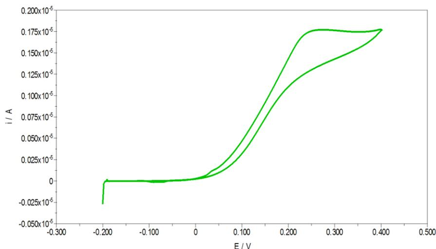
**Figure 4.13** Cyclic voltamograms of modified SPE with GO/PAH/DI towards 2 mM NADH and 35  $\mu\text{M}$  PAP. Scan rates 2.5 mV/s.
