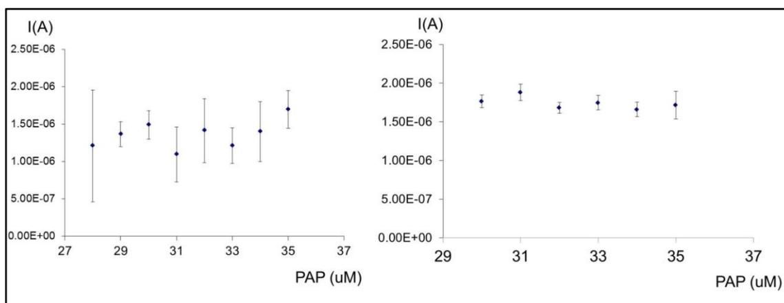
**Figure 4.15** Plot of the catalytic plateau current obtained at GO/PAH/DI modified SPE, 2  $\mu\text{L}$  and 5  $\mu\text{L}$ , as a function of of PAP concentration. NADH concentration was in excess of 2 mM in PBS buffer (pH 7.0). Scan rate: 2.5 mV/s.
