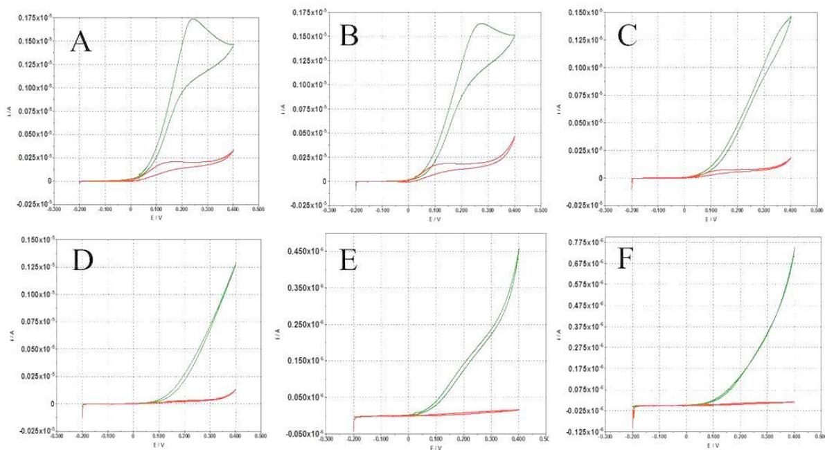
**Figure 4.12** Cyclic voltamograms of bare SPE (red) and modified SPE with GO/PAH/DI (green) towards 2 mM NADH with various concentration of PAP, 40,20,10,5,2.5,1  $\mu\text{M}$ , (A-F), respectively. Scan rates 2.5 mV/s.
