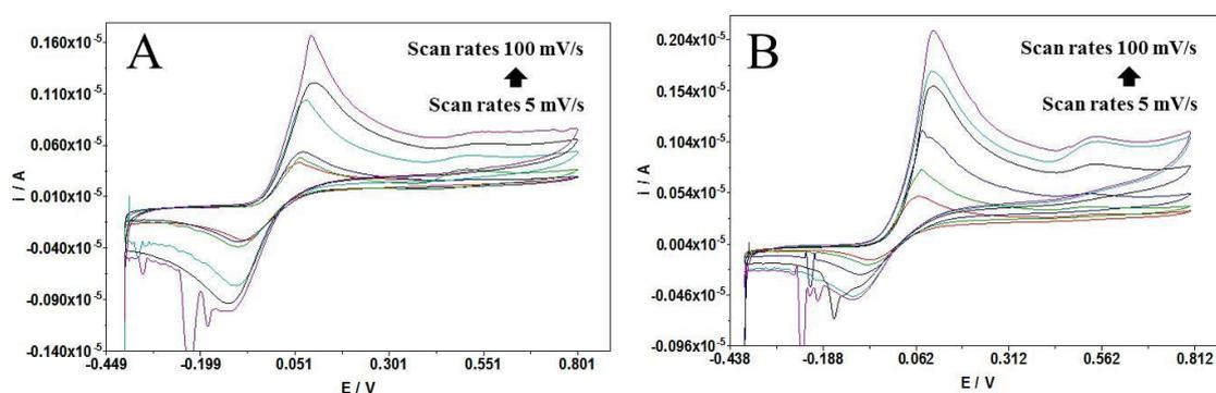
**Figure 4.9** Voltammograms obtained at different scan rates (from inner to outer): 5,10, 20, 50, 80, 100 mV/s. in 0.1 M PBS buffer (pH 8.0) containing 0.1 mM PAPP, 1 mM NADH and 10 unit of ALP (A) and 10 unit of ALP with DI (B)
