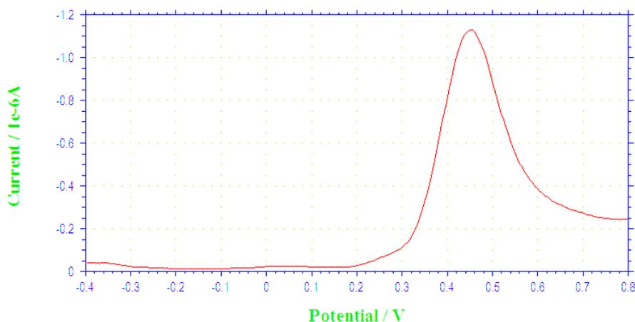
**Figure 4.17** DPV of response of (GO/PAH/ALP/DI)<sub>4</sub> label (fixed amount in microplate) towards 0.1 mM PAPP and 0.1 mM NADH . Scan rate 20  $\text{mV s}^{-1}$  and 2 min incubation time.
