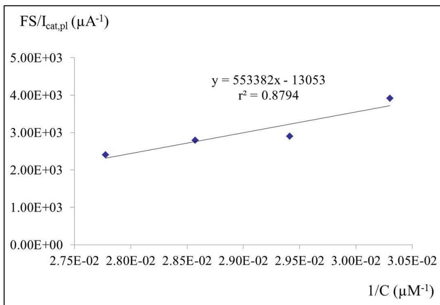
**Figure 4.14** Plot of the reciprocal of the catalytic plateau current obtained at GO/PAH/DI modified SPE as a function of reciprocal of PAP concentration. NADH concentration was in excess of 2 mM in PBS buffer (pH 7.0). Scan rate: 2.5 mV/s.
