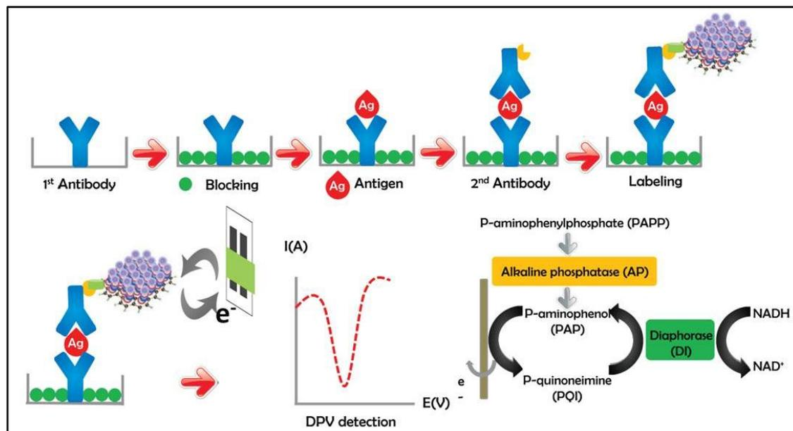
**Figure 4.3** Depiction of electrochemical immunoassay using (GO/PAA/ALP/DI)<sub>n</sub> labels on micro well plate.
