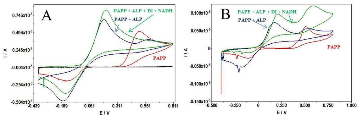
**Figure 4.6** Cyclic voltammograms obtained in 0.1 M PBS containing 0.1 M KCl pH 7.0 scan rate 50 mV/s. **A**; 1 mM pAPP (red) 1 mM pAPP with 10 unit of ALP (blue) 1 mM pAPP and NADH with 10 unit of ALP and 10 unit of DI (green). **B**; 0.1 mM pAPP (red) 0.1 mM pAPP with 10 unit of ALP (blue) 0.1 mM pAPP and NADH with 10 unit of ALP and DI (green)
