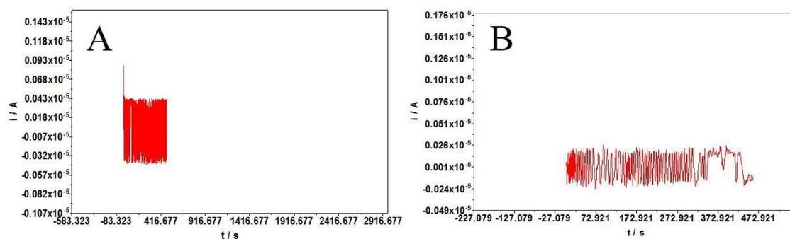
**Figure 4.8** Amperometric response of ALP and DI modified (drop-dried) SPEs electrode with successive injection of 2  $\mu\text{M}$  (left) and 20  $\mu\text{M}$  (right) pAPP at an applied potential 0.2V. in 0.5 M PBS buffer containing 0.1 M KCl pH 8.0 with stirring.
