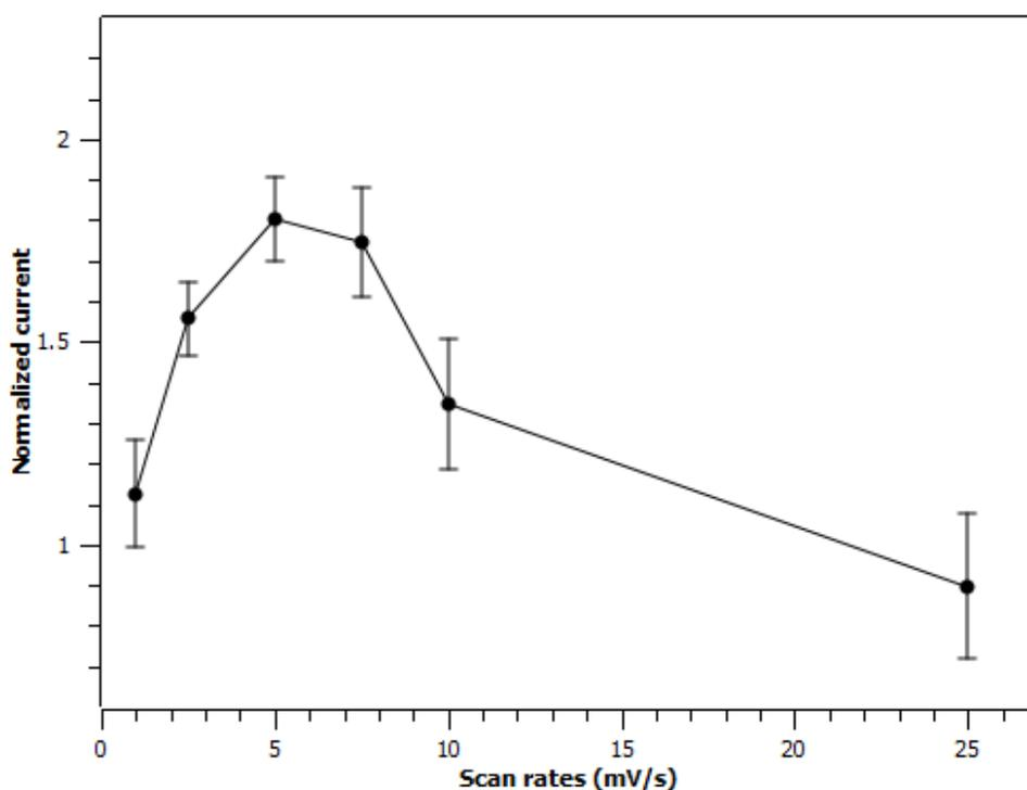
**Figure 3.19** DPV peak heights generated by MWNT-[PAH/Tyr]<sub>2</sub> labels incubated in microwell plates with 10 mM catechol for 2 mins before measurement. Currents are normalised relative to the peak current in the absence of enzyme at the relevant scan rate.
