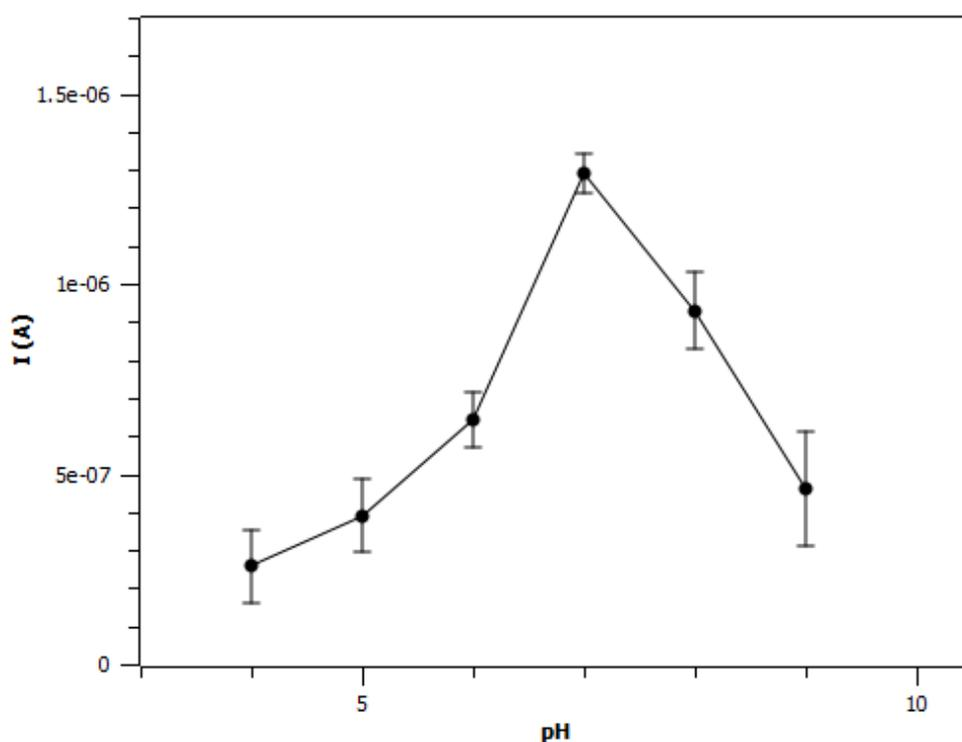
**Figure 3.13** Amperometric response of Tyr-MWNTs to various pH working solutions ranging from 4-9. Amperometry was conducted under 0.5 M PBS buffer containing 0.1 M KCl in different values of pH, under stirred conditions.
