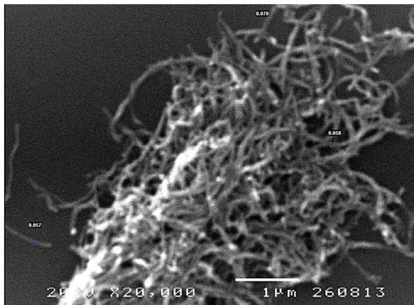
**Figure 3.7** SEM image of unmodified MWNT(3).
