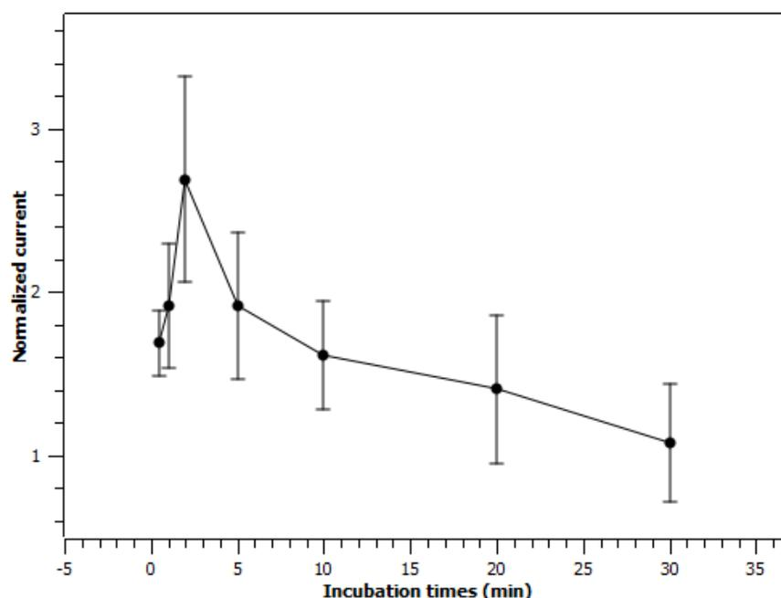
**Figure 3.18** Differential pulse voltammetric (DPV) peak heights generated by MWNT-[PAH/Tyr]<sub>2</sub> labels incubated in microwell plates with 10 mM catechol for varying periods before measurement. Currents are normalised relative to the peak current in the absence of enzyme. DPV conditions: Step potential = 0.6 mV, pulse interval = 0.125 s, modulation amplitude = 0.05 V.
