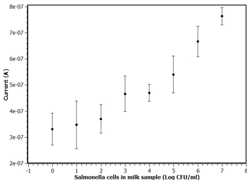
**Figure 3.21** Current response of *Salmonella* Typhimurium detection in milk sample using electrochemical enzyme labeling (error bars represent 3 replicate experiments).
