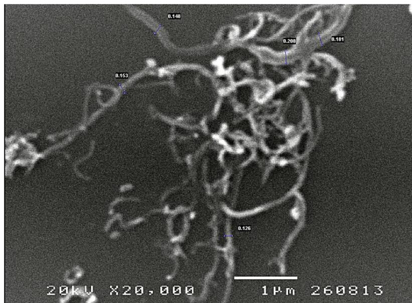
**Figure 3.9** SEM image of MWNT modified by two [PAH/Tyr]<sub>n</sub> bilayers (2).
