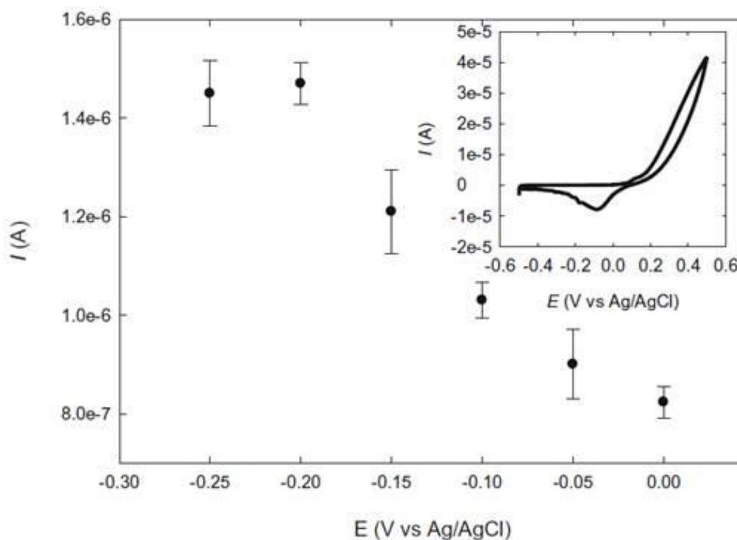
**Figure 3.12** Hydrodynamic voltammogram for the response of MWNT-[PAH/Tyr]<sub>2</sub> - coated screen printed electrodes to 4.0 μM catechol. Error bars show  $\pm 1$  stdev (n = 3). Each determination was made with a different electrode.
