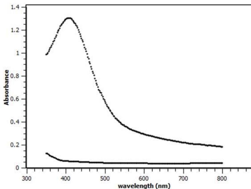
**Figure 3.22** The absorbance of benzoquinone (dot line) at 410 nm, a product from the reaction between tyrosinase enzyme and catechol, compare with the absorbance of catechol without tyrosinase (solid line).
