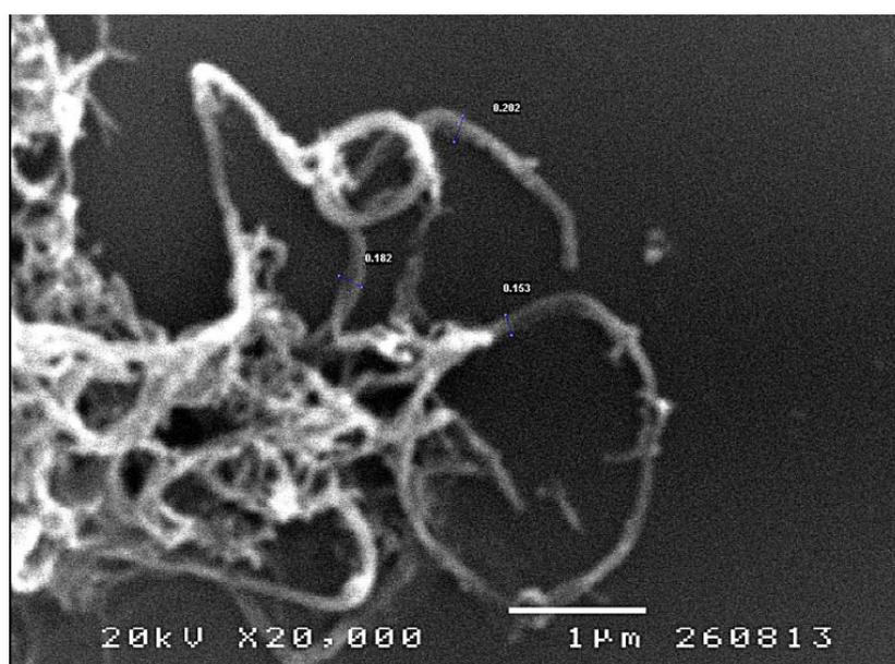
**Figure 3.10** SEM image of MWNT modified by two [PAH/Tyr]<sub>n</sub> bilayers (3).
