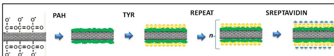
**Figure 3.2** Depiction of layer-by-layer electrostatic self-assembly of Tyr on MWNTs.
