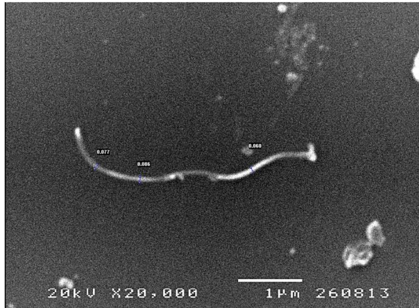
**Figure 3.5** SEM image of unmodified MWNT (1).
