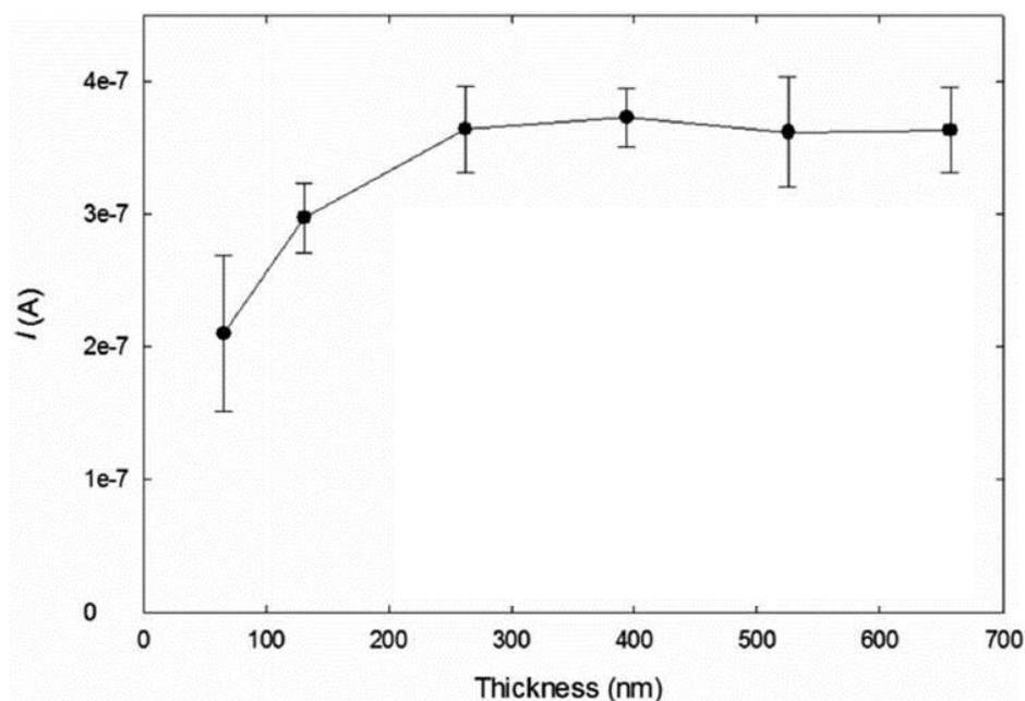
**Figure 3.16** Amperometric response to 4.0  $\mu\text{M}$  catechol at -0.20 V vs Ag/AgCl using screen printed electrodes modified by MWNT-[PAH/Tyr]<sub>2</sub> coatings of varying film thickness (nm).
