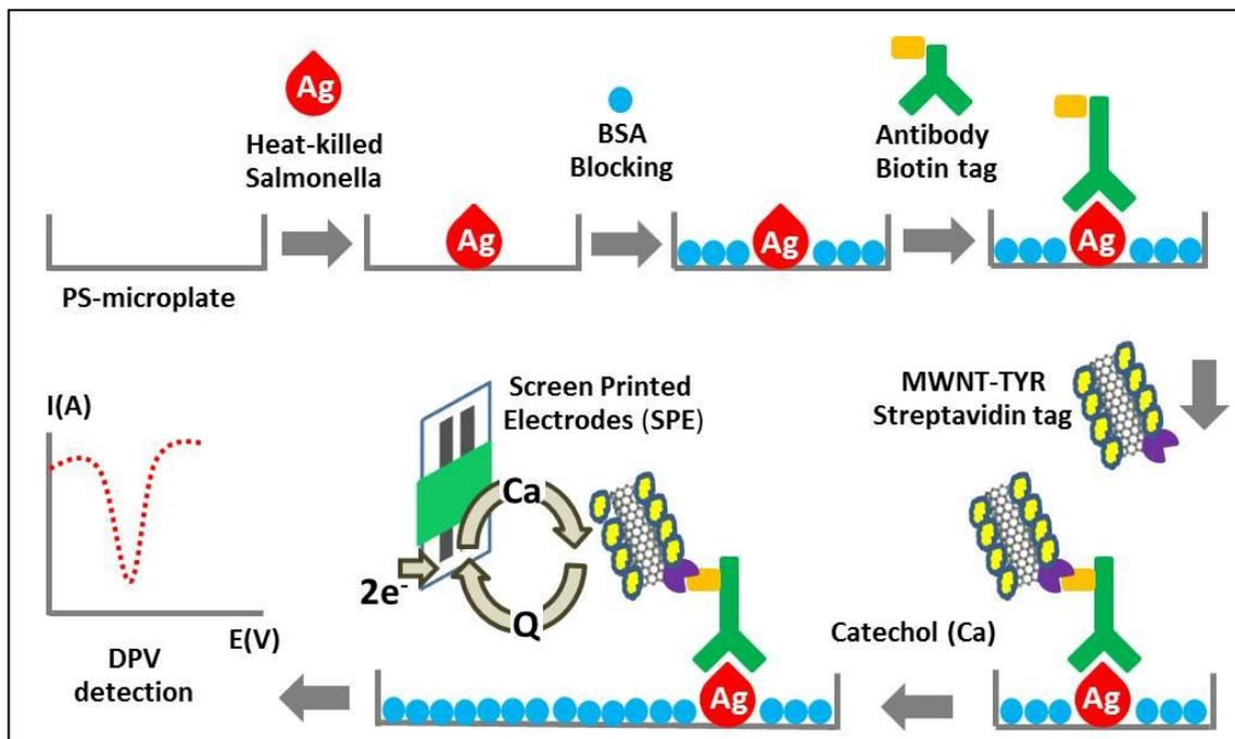
**Figure 3.3** Depiction of electrochemical immunoassay using  $(\text{MWNTs/PAH/Tyr})_n$  labels on micro well plate. Ag, Ca, Q represent antigen, catechol and quinone, respectively.
