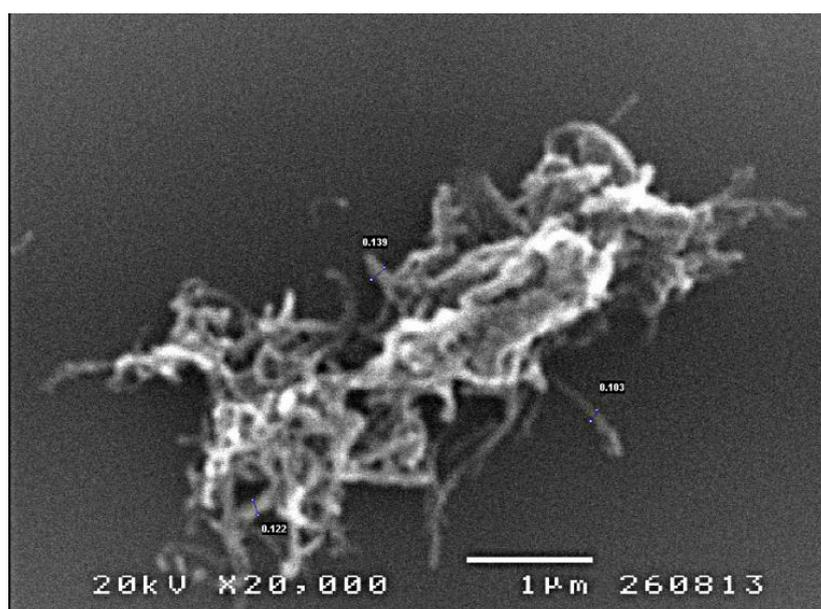
**Figure 3.8** SEM image of MWNT modified by two  $[\text{PAH}/\text{Tyr}]_n$  bilayers (1).
