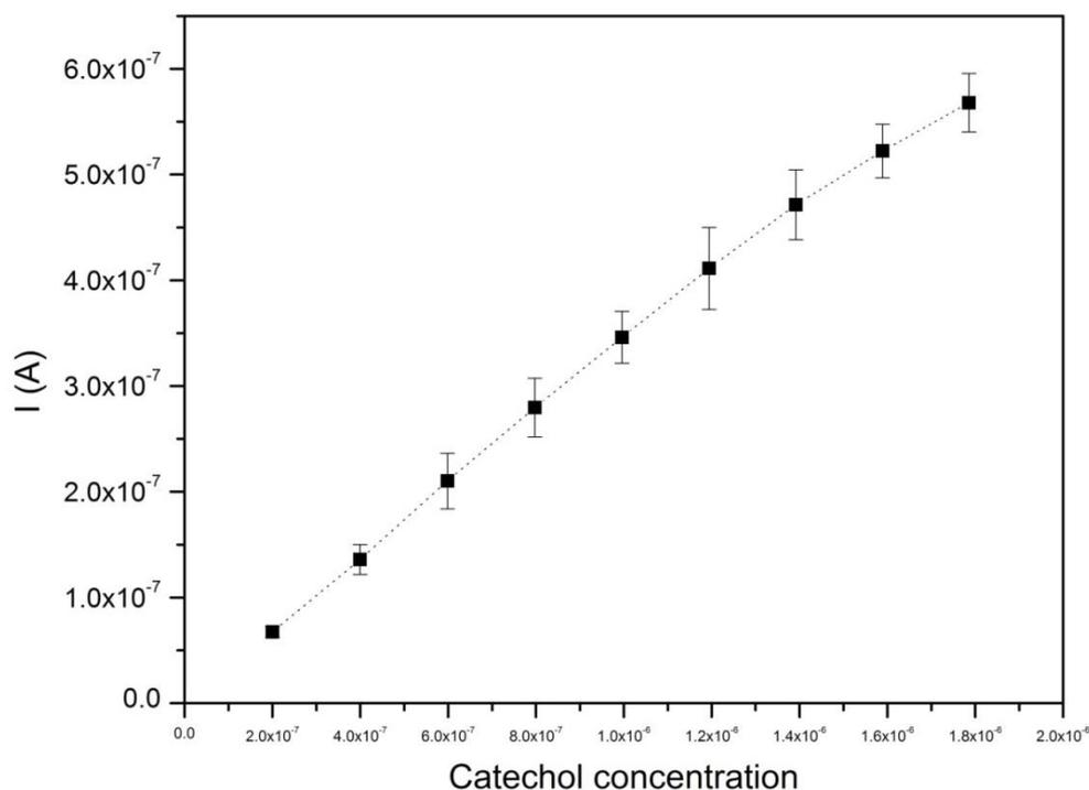
**Figure 3.15** Linear response of MWCNTs/PDDA/Tyr<sub>2</sub> for catechol. Experimental condition: 0.2  $\mu\text{M}$  of catechol, 0.1 M PBS + 0.1 M KCl, potential -0.2 V.
