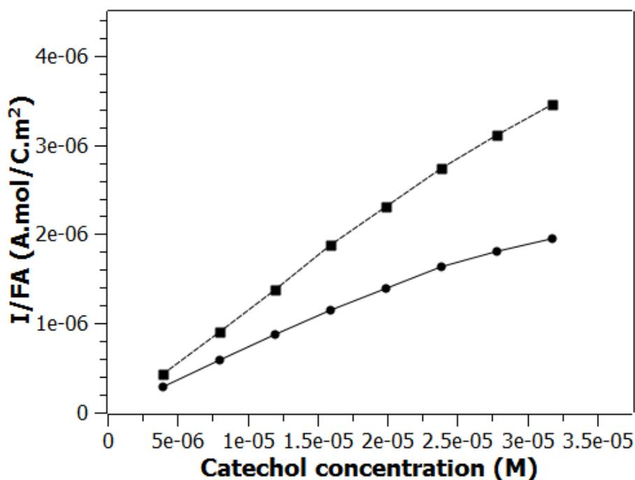
**Figure 3.17** Calibration of catechol using MWNT-[PAH/Tyr]<sub>2</sub> films of 390 nm and 60 nm.
