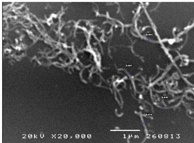
**Figure 3.6** SEM image of unmodified MWNT (2).
