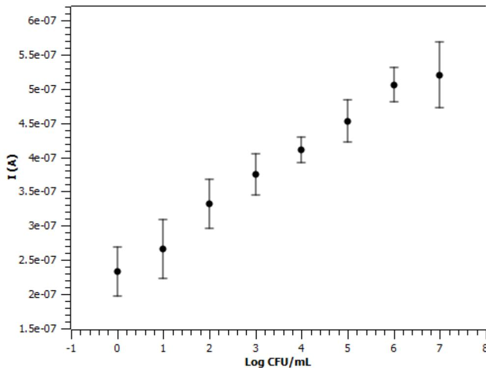
**Figure 3.20** DPV determination of heat-killed *Salmonella* Typhimurium (scan rate =  $5 \text{ mV s}^{-1}$ ) by direct ELISA using MWNT-[PAH/Tyr]<sub>2</sub> labels incubated in microwell plates in the presence of 10 mM catechol for 2 mins.
