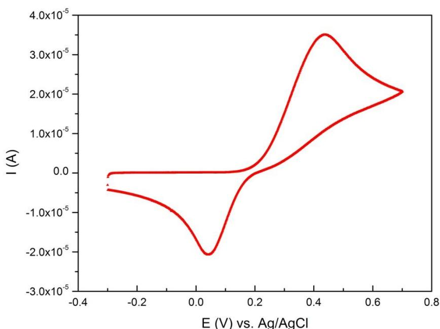
**Figure 3.11** Cyclic voltammogram of 5 mM catechol solution in PBS pH 7.0 containing 0.1 M KCl. The voltametry was made at  $50 \text{ mV}\cdot\text{s}^{-1}$  using a glassy carbon electrode (BAS).
