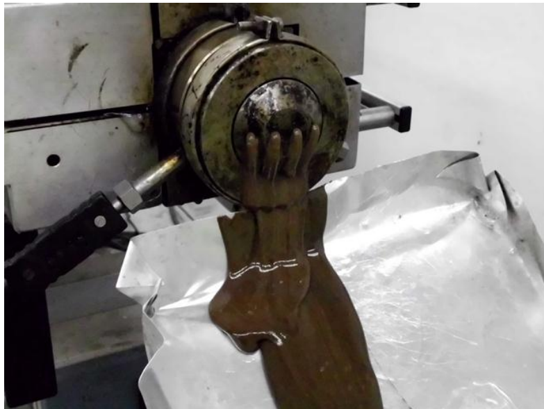
Figure 3.10 Over-melted wood/PLA loaded with 1.5%wt Zeomic composites during the extrusion process
