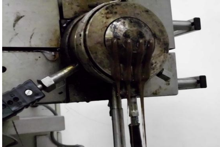
Figure 3.6 Over-melted PLA loaded with 20 and 40 %wt wood flour during the extrusion process
