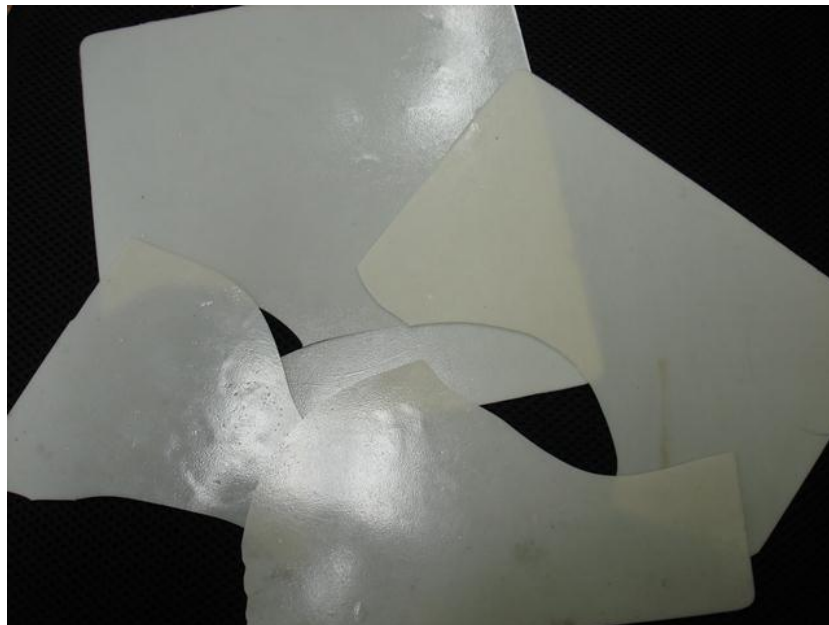
Figure 3.9 Broken Zeomic/PLA composite sheets
