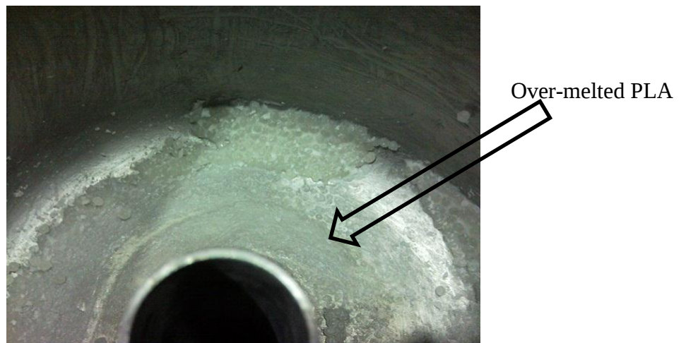
Figure 3.5 Over-melted PLA during the high speed mixing process
